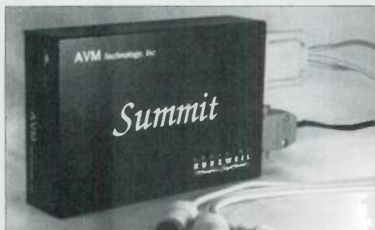
AVM Technology's Summit is a free-standing synth module that uses the Kurzweil MASS chip set. Originally designed for use with PC sound cards, the black metal box can also be used with a Macintosh.
