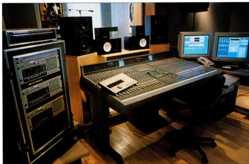
A rack of TASCAM DA-88s designed by the author is ready to transfer tracks at D'Elia Wittkofski post-production studios in Pittsburgh, Pennsylvania.
