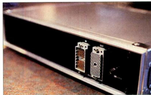
FIG. 2: The EDAK/ELCO connectors on the remote patch facility facilitate quick setup. The I/O of the three DA-88s in the mobile rack can be completely hooked up with just two connections, rather than plugging in 48 separate cables.
