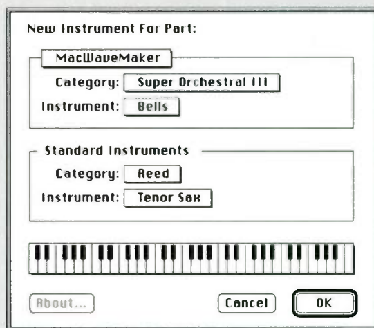
FIG. B: Sample Instrument Picker screen during conversion of a MIDI file to QuickTime movie, using a prototype MacWavemaker driver that supports access to all ROM sound banks. If played on a Mac without MacWavemaker, QuickTime substitutes a Tenor Sax from its default General MIDI sound set in place of the Bells.
