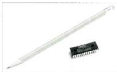
FIG. 1: The HDCD decoder can be implemented in a small, inexpensive chip for mass production.
