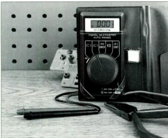
A digital multimeter (DMM), such as this Micronta unit from Radio Shack, can be used to check suspect fuses and to measure AC adapter output. However, keep in mind that under no-load conditions the AC adapter measurement may be misleading.
