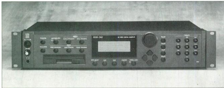
The E-mu ESI-32 packs a lot of sampler into a 2U rack-mount box, including 32-voice polyphony, up to 32 MB of RAM, resonant filters, and an intuitive user interface.
