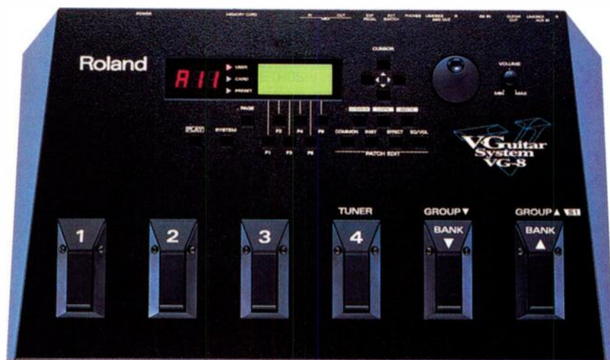
The Roland VG-8's main unit is housed in a sturdy metal case. The pedals let you select among three Groups of 64 Programs each, and the LED and LCD displays are bright.
