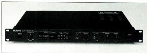
FIG. 4: Roland's SN-550 applies downward expansion to five frequency bands independently and includes hum cancellation.
