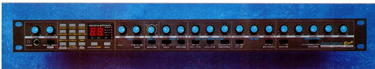
The monophonic BassStation Rack offers real-time MIDI modulation, ample presets, and potent analog-synth bass and lead sounds.
