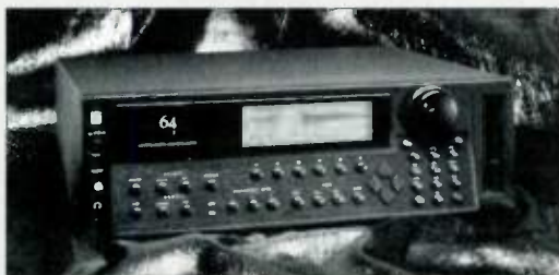
E-mu's e-64 is essentially a budget EIV with half the polyphony and RAM capacity.
