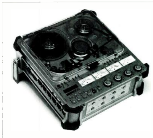
The 4-track Nagra-D digital audio deck used for the Lieberman project records at 24 bits per sample onto standard, 1/4-inch metal oxide tape.
