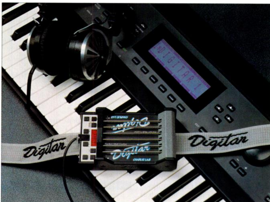
By revoicing MIDI notes to sound like they were picked or strummed on a 6-string guitar, Charlie Lab's Digitar can make a keyboardist sound like a guitarist.
