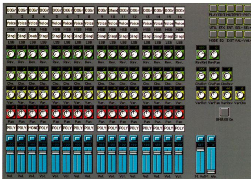
FIG. 1: Because of the MU80's small display and numerous hidden parameters that can only be addressed via SysEx, you may prefer to program it with a custom template such as this mixer screen from EMAGIC's Logic sequencer.
