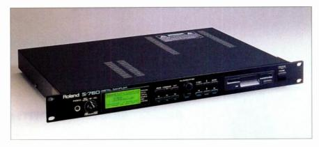
The Roland S-760 does a great job converting S1000 sounds, the only non-Roland format it supports. Because of the sampler's emphasis/de-emphasis scheme, some converted samples display a slight high-frequency rolloff.
