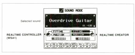
FIG. 3: The Sound Mode display includes the name of the Sound, the Realtime Controller and Creator assignments, and various parameters along the bottom. (Courtesy Technics.)
