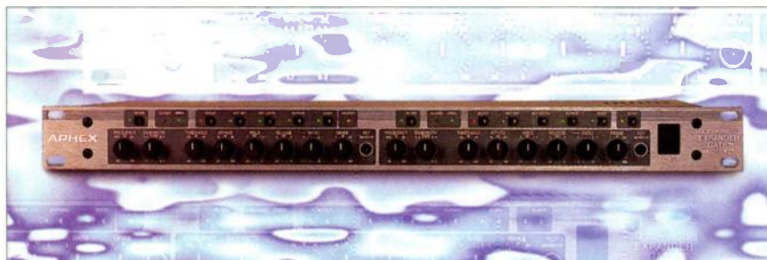
The full-featured front panel of the Aphex 622 Logic Assisted Expander/Gate provides a key-listen button for studio monitoring and a key-monitor jack for listening to the sidechain during live-sound applications.
