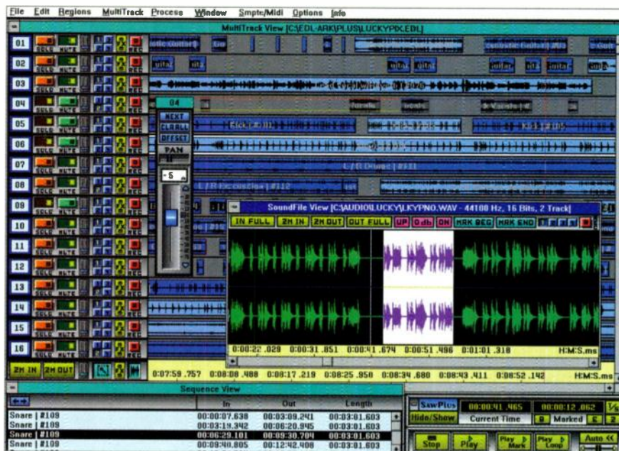
FIG. 2: Innovative Quality Software's SAW Plus lets you record and edit more audio tracks than any other Windows program that uses standard Windows sound cards.
