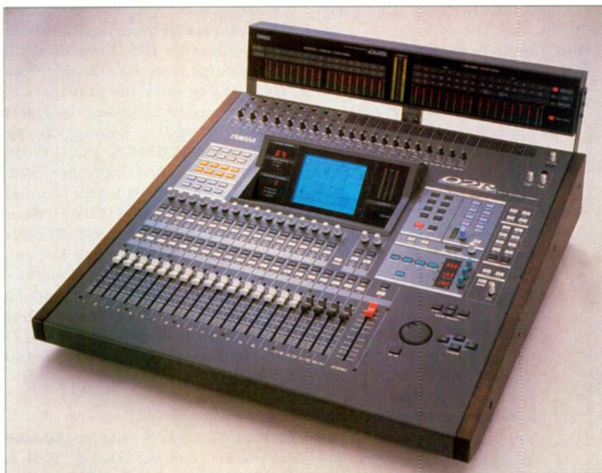
Yamaha's 02R digital console is probably the most revolutionary recording product for project studios since the Alesis ADAT. This fully automated mixer features extensive digital I/O and oodles of onboard effects, dynamics processing, and parametric EQ.
