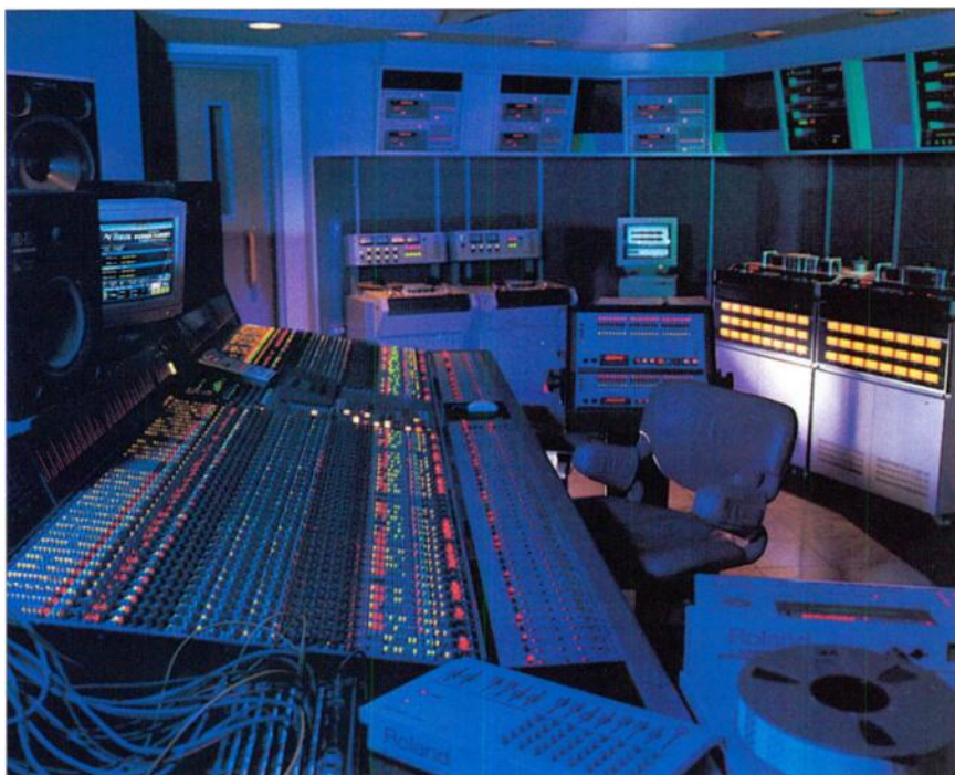
The main control room in this studio at Full Sail features a Neve VR60 console, two 24-track Otari MTR-100s, three 8-track TASCAM DA-88s, and a Meyer 2000-watt monitoring system.
