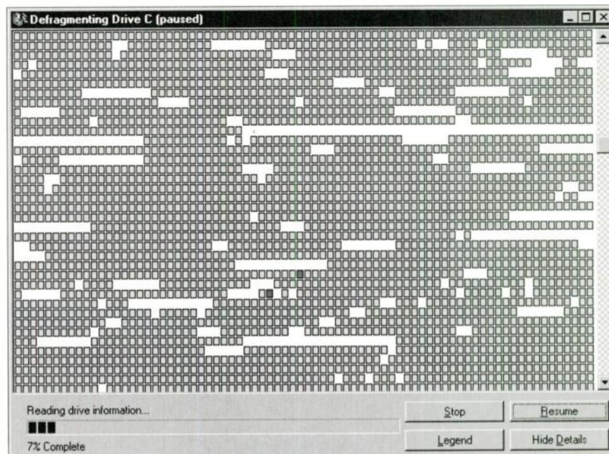
FIG. 2: This section of a drive is fragmented. The blank areas represent blocks that contain no data. These gaps were created when the data located in those blocks was changed or deleted.
