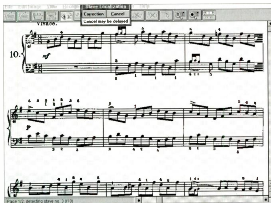
FIG. 2: During recognition, PianoScan steps through each staff one symbol at a time.
