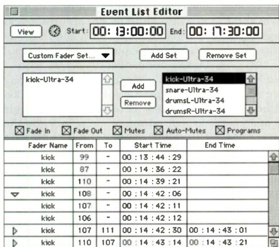
FIG. 4: The Event List Editor contains all of the fader, mute, automute, and Program Change data recorded in your current session. Clicking on check boxes determines what events are displayed, and custom Fader Sets can be created when editing selected channel groups.
