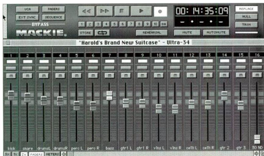
FIG. 1: All recording functions are available from UltraMix Pro's Transport window and from the UltraPilot Control Interface. Fader resolution can be changed by clicking on the buttons in the lower-left corner of the Fader window. Subgroups are designated by the different colors of the individual faders.
