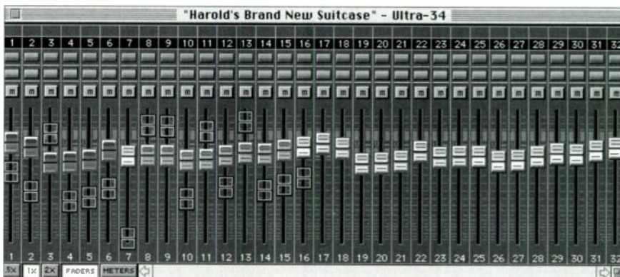
FIG. 3: With fader resolution set at 1x, 32 channels are visible on a 14-inch monitor. The clear "glass" faders show the actual positions of the UltraPilot faders in relation to the recorded fader locations.
