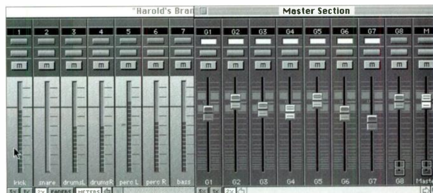
FIG. 2: Clicking on the Meters button in the Fader window (left) changes the faders to peak meters that display audio activity for each channel. The Master window (right) contains controls for each of the eight subgroups and the master bus.
