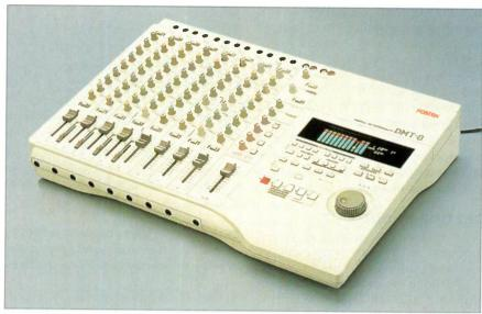
Fostex's DMT-8 is clearly aimed at the cassette Multitracker user. It's the only M-HDR with an analog mixer, and it lacks many professional features. But it sounds very good, and it is the least-expensive 8-track M-HDR.
