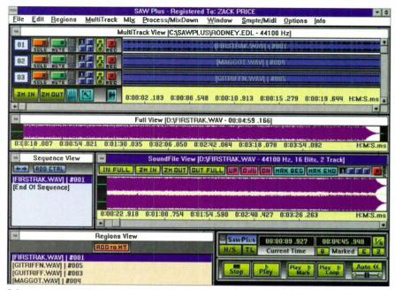
FIG. 1: SAW Plus' default main screen, at 800 x 600 resolution, shows the Multitrack, Full View, Soundfile, Sequence, and Regions windows plus the playback transport controls.
