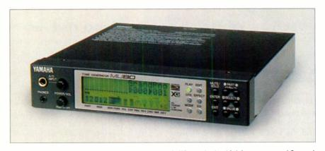
The MU80 64-voice tone module introduced Yamaha's XG standard, which is a superset of General MIDI. Most of the module's parameters can be programmed from the front panel, but some can only be accessed via SysEx.
