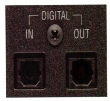
FIG. 5: The Alesis ADAT uses a proprietary optical interface called the Lightpipe.
