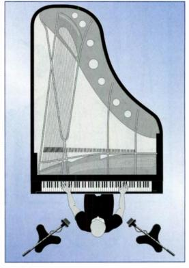
FIG. 2: Placing the microphones on either side of the player position produces a realistic, stereo effect.
