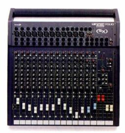
The Folio SX also offers a headphone jack; insert points for the main mix; switchable, global, +48V phantom power; and 2-track returns on RCA jacks. Two 3-color, 10-segment bargraph LED meters can be switched to show mix output, PFL, or AFL solo levels. A latched power connector ensures that the detachable power cord remains secure.
