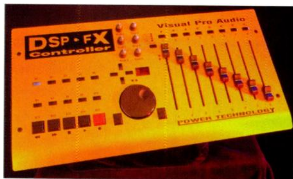
The DSP•FX Controller is a repackaged JLCoooper CS-102, which provides an excellent alternative to mouse control. However, you can use any MIDI fader box or sequencer to accomplish the same ends.
