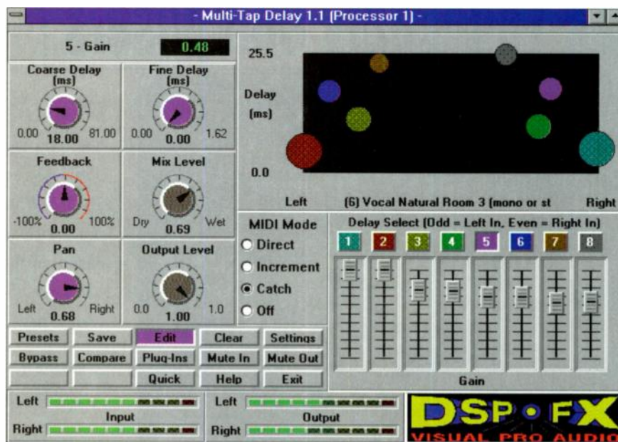
FIG. 2: This shot of the Multi-Tap Delay shows the virtual controls for the fifth delay tap and the graphic display of all eight taps and their relative settings.
