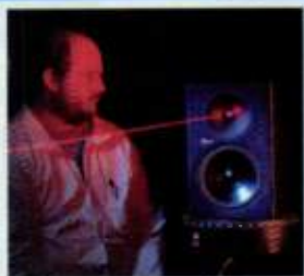
Meddie acoustic engineer David Bie uses scanning laser vibrometry to map HR824 tweeter dome vibrations. Film at 11.
