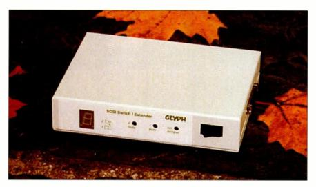
Glyph Technologies' GSS-210S SCSI Switch/Extender allows you to switch your computer between two sets of SCSI devices and extends the SCSI chain's maximum length.
