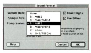
FIG. 3: SoundEdit 16 2.0 offers MACE compression and Macromedia's compression algorithm for 8-bit sounds as well as IMA/ADPCM and µLaw compression for 16-bit sounds.
