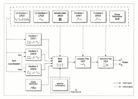
FIG. 1: The Pulse's voice architecture will be familiar to veteran analog-synth users. Components enclosed within the dotted box at the top are modulators. The optional Pulse Plus audio input is shown in the dotted box at the bottom. All other components are in the regular audio path. (Courtesy Waldorf)
