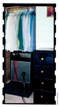
FIG. 7: A closet crammed with loads of clothing provides considerable sound absorption for capturing a dry, very present bass-guitar signal. This Harmony 525 bass amp is miked with an AKG D 112 dynamic mic.
