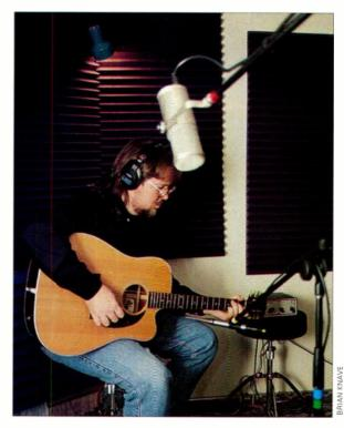
FIG. 2: You can create a more complex stereo picture of the acoustic guitar by using two different mics. Here, an Earthworks OM1 is aimed just below the strings to capture sparkle and attack from songwriter Mike Lawson's Gibson J-30C, while a Rode Classic, set to omni, reproduces the broader, ambient sound of the guitar.
