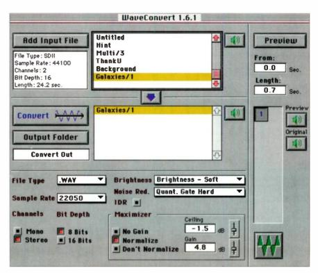
FIG. 6: WaveConvert offers several audio-processing options to improve the results of downsampling and 16-to-8-bit reduction. Sophisticated algorithms maximize sound quality during conversions between file formats.
