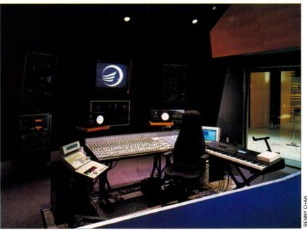
In this room designed by George Neuberg of Studio 440, note how symmetrically the mix position has been laid out. Consistent elements on the right and left help maintain proper stereo imaging.
