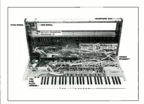
The Moog Memorymoog. The upper cab is open in service position, prior to calibration.
