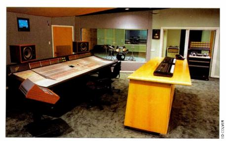
Pro studios, such as the L.A. Recording Workshop in North Hollywood, employ a machine room (visible behind the keyboard station) to prevent noise from invading the control room. Desktop recordists can modify a closet to silence their disk drives. (Courtesy studio bau:ton)
