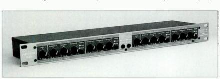
The Model 109 incorporates Aphex's sweet-sounding Tubessence hybrid tube technology into a flexible, 4-band parametric EQ. You can use all four bands on one channel or switch the unit to dual mono with two bands per channel.
