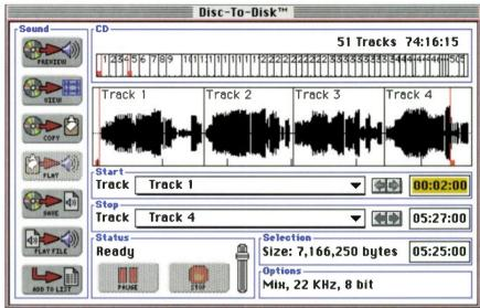
FIG. 5: OMI's Disc-To-Disk uses a colorful graphic interface that shows the contents of CD tracks as waveforms. You can select part of a track or several tracks and convert the selection to any of five file formats.
