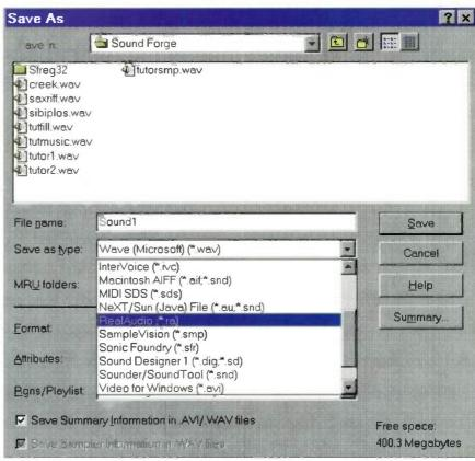
FIG. 4: The Save As dialog box in Sonic Foundry's *Sound Forge* 4.0 includes a drop-down menu with eighteen file formats from different computer platforms.
