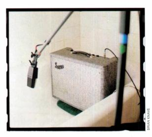
FIG. 2: The sound of a cranked-up Supro tube amp is given a dose of attitude and reverb by being recorded in a bathtub.
