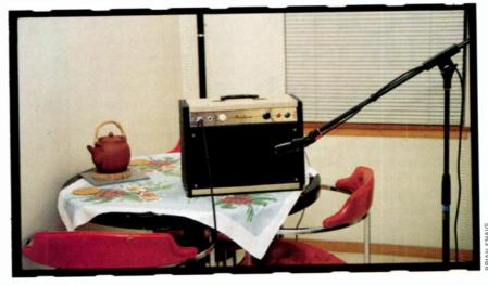
FIG. 6: The numerous reflective surfaces in a kitchen lend glorious reverb to the sputtering chaos of an overdriven tube amp. Here a Shure SM57, angled off-axis, documents the rattling of the tiny Jensen speaker in a vintage Airline amp while an AKG C 414 in omni mode (not shown) captures the room tone from fifteen feet back.
