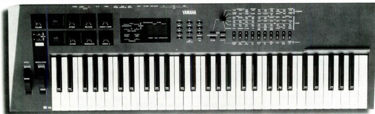
Yamaha's CS1x keyboard synth offers real-time parameter control via front-panel knobs. It incorporates the synthesis engine from the company's popular MU50 synth module and includes a special bank filled with fat, analog-like sounds.
