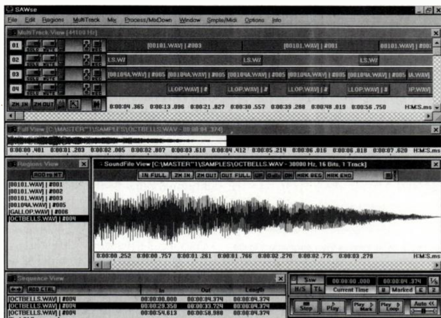
FIG. 2: SAW SE's Multitrack window (at the top of the screen) shows digital audio regions arranged along a timeline.
