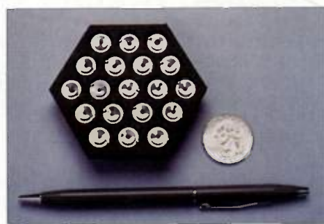
FIG. 1: The original HSS emitter consisted of several piezo mic elements arranged in a hexagonal array. (Courtesy ATC)
