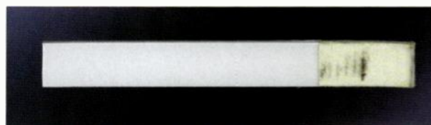
FIG. 2: The dark lines on this chamois swab show the dirt cleaned from an ADAT-XT head after 150 hours of operation.
