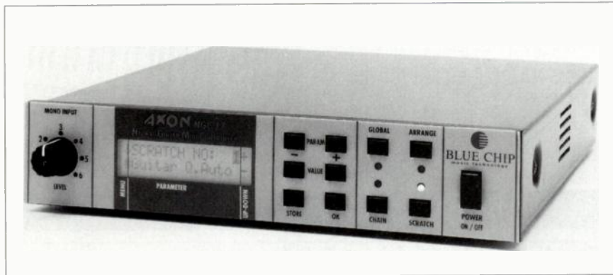
The half-rack Blue Chip Axon NGC 77 uses neural-network technology to reduce tracking delays when converting notes played on a guitar into MIDI information.
