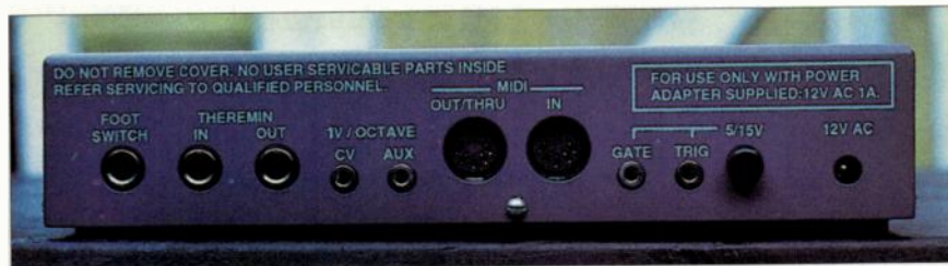
FIG. 3: The MIDI-Wave sends gate and trigger signals when the amplitude reaches a selectable threshold, which can be set to 5V or 15V using a rear-panel switch (lower right). The MIDI Out/Thru port's function is software selectable.
