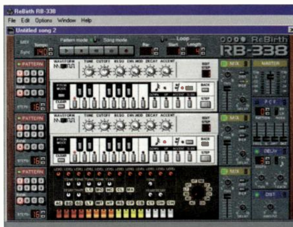
FIG. 1: ReBirth RB-338 emulates two Roland TB-303 synths and a TR-808 drum machine, and it adds an extra envelope-controlled filter, delay, and distortion effect.
