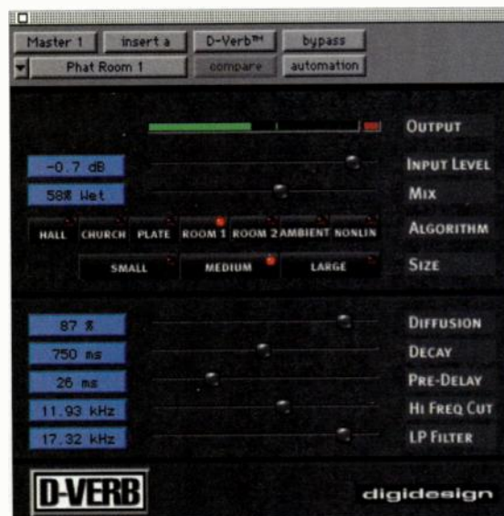
FIG. 1: Digidesign's versatile D-Verb TDM plug-in offers a clean, easy-to-use interface.
