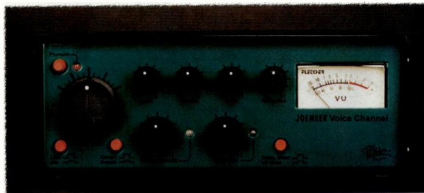
Joemeek's Voice Channel combines a mono mic preamp, a compressor, an instrument preamp, a direct box, and a spectral enhancer.
