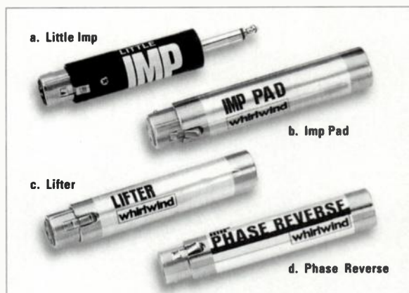
FIG. 2: Whirlwind’s Little Imp (a) is used for connecting low-impedance (low-Z) mics to high-Z inputs. The Imp Pad (b) comes in four models (10, 20, 30, and 40 dB) for attenuating balanced low-Z signals. The Lifter (c) lifts the ground by disconnecting pin 1, and the Phase Reverse (d) works by reversing pins 2 and 3.
