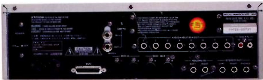
FIG. 1: The rear panel includes stereo audio inputs and main outputs, a headphone jack, a SCSI port, and two sets of MIDI In and Out jacks. Optional expansion boards can add S/PDIF digital I/O and eight more analog outputs as well as SMPTE sync I/O.
