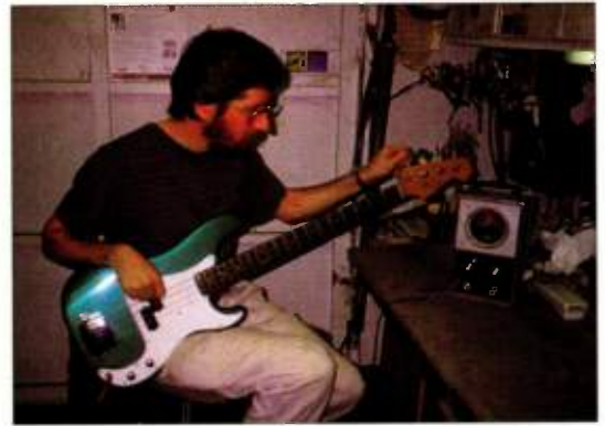
Luthier John Jordan has intonated hundreds of basses using his strobe tuner.
