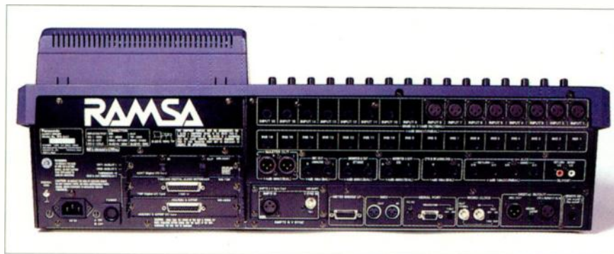
The DA7's top row of connectors includes XLR inputs for channels 1 to 8 and balanced, 1/4-inch inputs for channels 9 to 16. Row 2 holds the channel inserts, while row 3 contains the outputs and aux buses. The bottom row sports the meter-bridge port, MIDI ports, serial ports, word-clock I/O, digital Record Out, digital 2-track In, and the footswitch jack. The expansion slots are on the left.
