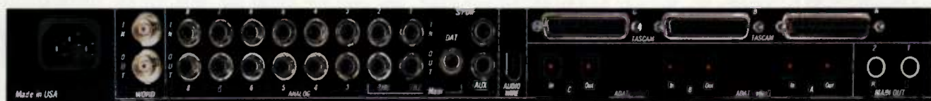
FIG 1 The 2408 audio interface offers a plethora of I/O. Up to three I/O boxes can connect to one PCI-324 card via a FireWire-style cable. Word-clock connectors are on the I/O box; ADAT 9-pin and MOTU Digital Timepiece sync ports are on the PCI card.
