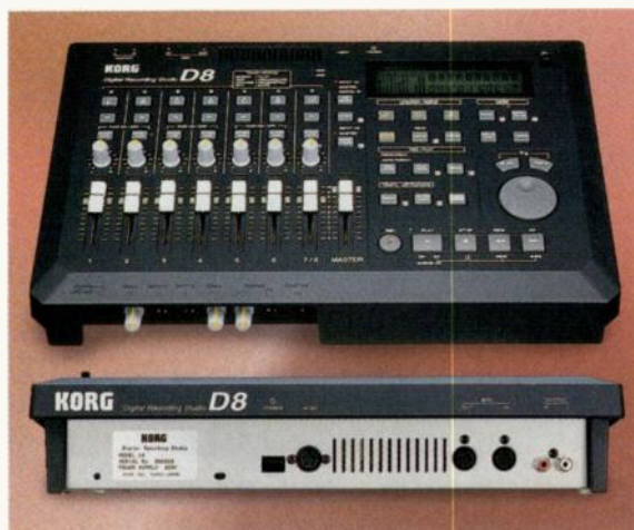
The Korg D8 is a great little songwriting tool, particularly for guitarists, thanks to its built-in drum patterns, tap-tempo feature, and guitar-oriented effects.
