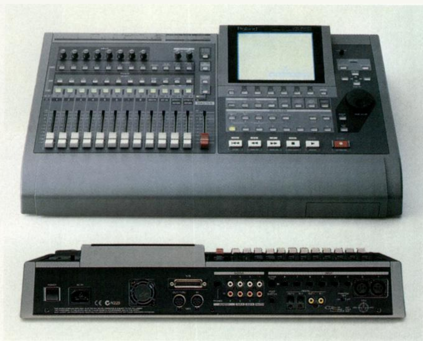
The current cream of the portable digital studio crop is the 16-track Roland VS-1680, with its huge graphic display, tremendous selection of built-in effects, advanced features, and flexible array of inputs and outputs. It has everything the VS-880EX offers and much more.
