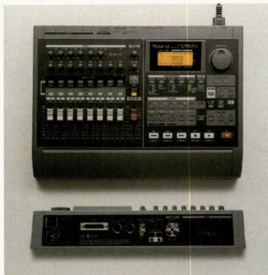
The Roland VS-880EX is the latest iteration of the product that really kicked this whole phenomenon into high gear. It includes a slanted, backlit display; EZ-Routing features; lots of virtual tracks; onboard automation; and a great-sounding effects processor.
