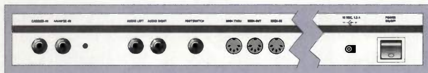
FIG. 1: In addition to its analog outputs, a footpedal jack, and MIDI ports, the Sirius's rear panel has two analog vocoder inputs, one for the carrier and one for the modulator (marked "Analyze-In"). A small knob allows you to adjust the gain of the Analyze input.
