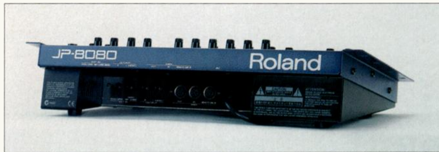
FIG. 2: The JP-8080's rear panel is recessed, so space is left for cables when you rack-mount the unit. In addition to the two audio inputs at the lower left, the JP-8080 has a front-panel mic input. When the front input is active, the rear inputs are off. Note the onboard power supply—no wall warts here!
