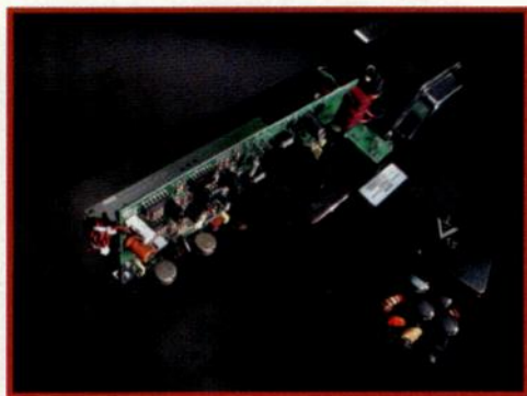
FIG. 4: Velodyne Silicon Systems' Class D amps can be much smaller than more conventional designs.
