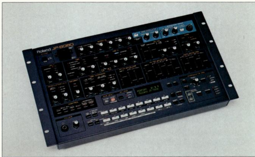
The Roland JP-8080 is absolutely loaded with sound- and phrase-creation features, audio-manipulation tools, and assorted bells and whistles. This is not your average analog-modeling synth; it's a fascinating instrument that requires no MIDI keyboard, although it can certainly be played conventionally.
