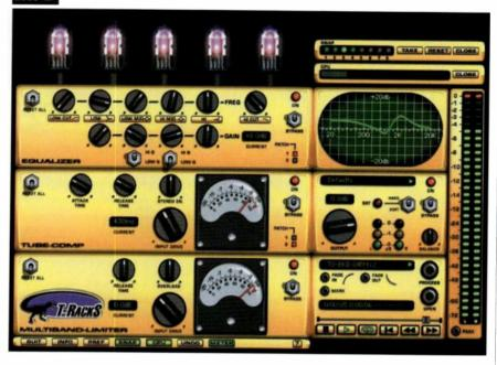
FIG. 4: IK Multimedia's T-Racks stereo mastering software features a 6-band parametric equalizer, a compressor, a multiband limiter, and a stereo enhancer. The program emulates the sound of vacuum-tube gear.
