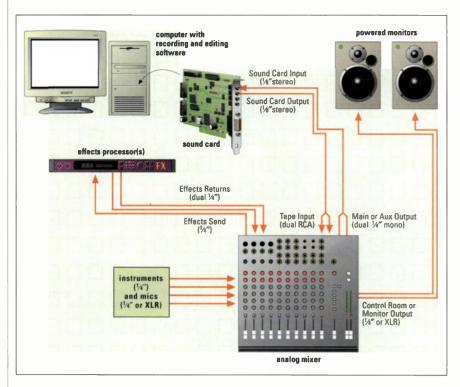
FIG. 2: This simple desktop music setup is surprisingly powerful. But the mixer requires a special feature—tape inputs—to make it work.
