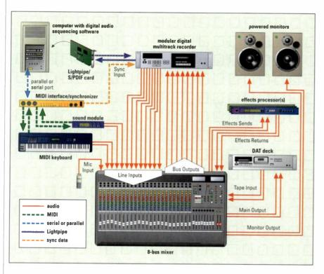
FIG. 5: By connecting a digital tape recorder to a computer and an 8-bus mixer, you can record and edit digitally but mix in the analog domain.
