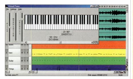
FIG. 3: The Virtual Piano applet is included with Cakewalk's Windows sequencers to facilitate note entry when no MIDI device is available. The computer keys that trigger the notes are shown beneath the piano keyboard display.
