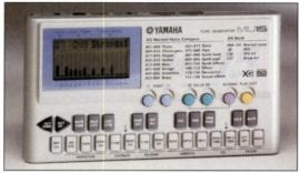
FIG. 2: Yamaha's MU15 synth is made to order for mobile music production. Featuring 32-note polyphony and 16-part multitimbral operation, the MU15 can connect directly to a notebook's serial port.
