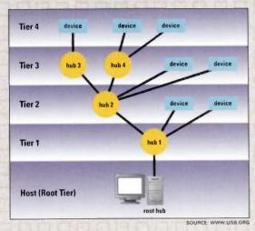
FIG. 1: A USB system includes one host (the computer) and a number of hubs and devices, arranged in a tree-branch or tiered-star configuration.
