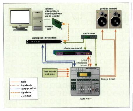
FIG. 6: Thanks to 8-channel digital audio interfaces, this powerful setup is a snap to hook up.
