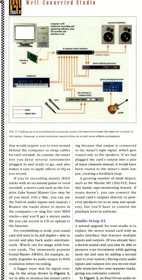
FIG. 3: Trading up to a multichannel computer audio interface eliminates the need for a mixer in this setup. However, a small submixer would allow us to add more effects processors.
