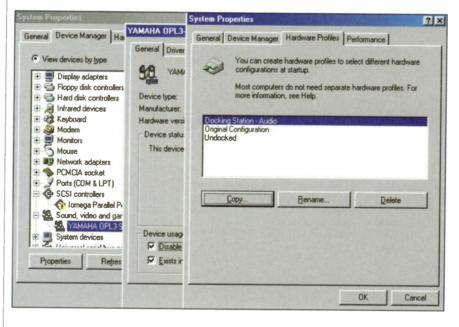
FIG. 8: Using the Windows Device Manager to disable his laptop's built-in audio, author Brian Smithers frees up an IRQ and two DMAs for use by the audio hardware attached to his docking station. This configuration can be saved as a Windows Hardware Profile.
