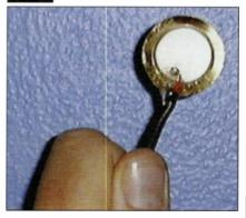
FIG. 2: A cheap, homemade contact mic can help you collect signature sounds.
