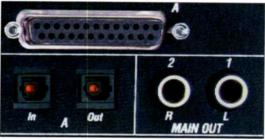
FIG. 4: This close-up of the MOTU 2408 audio interface shows 8-channel Lightpipe and TDIF connectors next to a 1/4-inch phone jack. The TDIF connector carries both incoming and outgoing signals.
