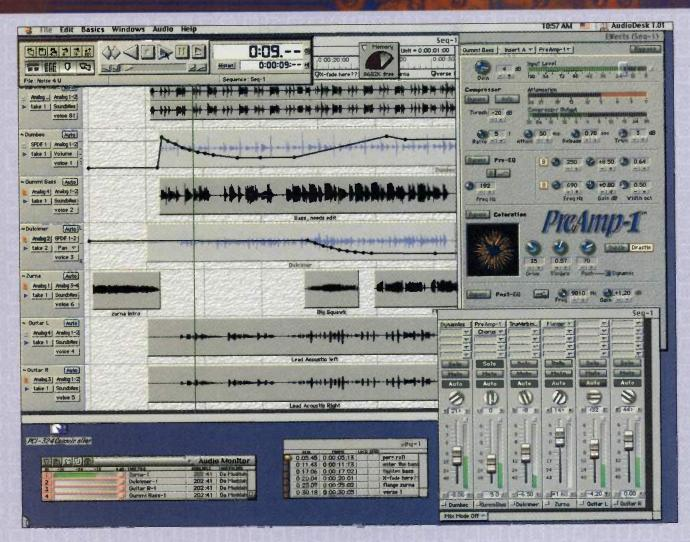
FIG. 1: MOTU AudioDesk (Mac) contains the main windows you'll find in most multitrack recording software. Clockwise from upper left: transport controls, disk-space gauge, plug-in effect controls, mixer, region markers, and record-level meters. At center is the tracks window.
