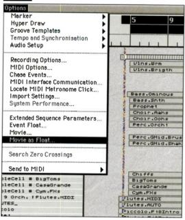
FIG. 1: When importing a QuickTime movie into Logic Audio, you have the option to display it in a window that will always stay on top.
