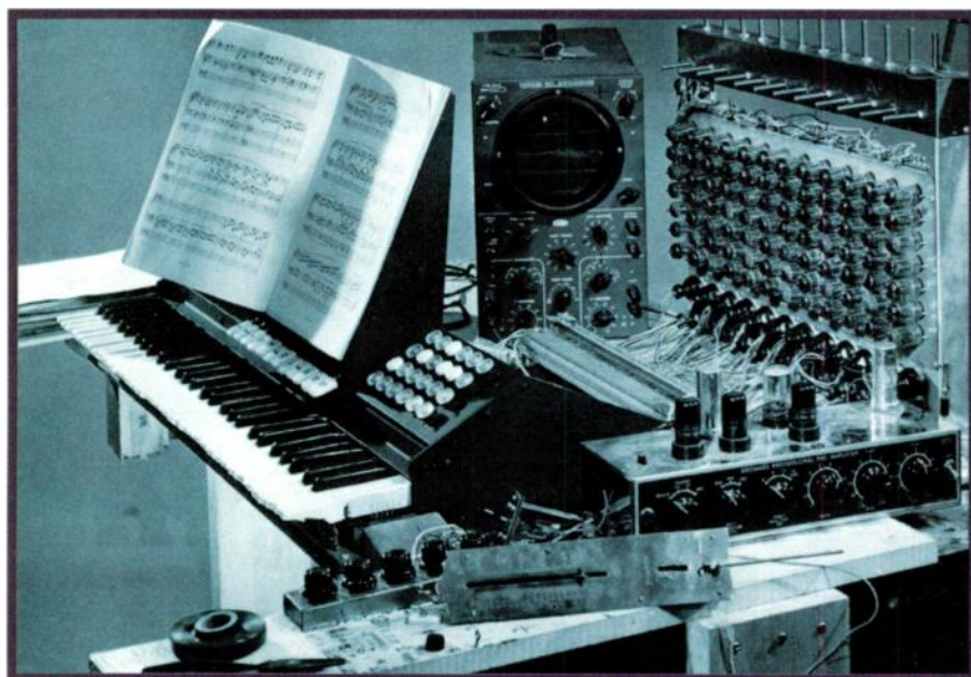
FIG. 11: A prototype Touch Sensitive Organ (1954) included a bank of vacuum-tube oscillators and an oscilloscope for viewing waveforms.
