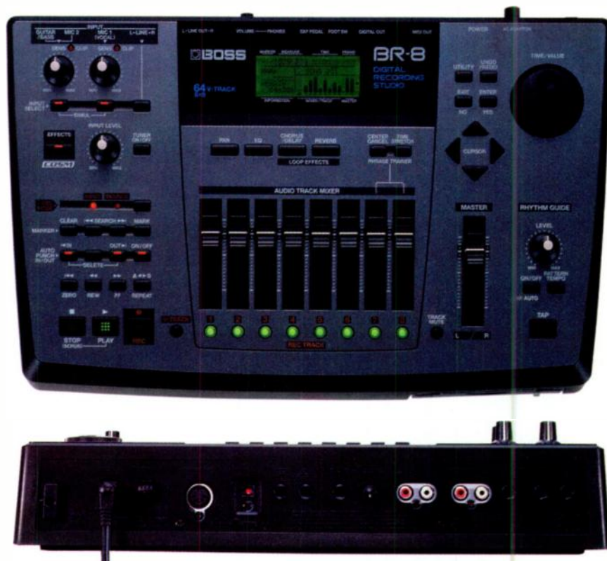
FIG. 1: The Boss BR-8 provides entry-level simplicity with great sound. The rotary dial lets you scrub audio, but the unit has no waveform display.
