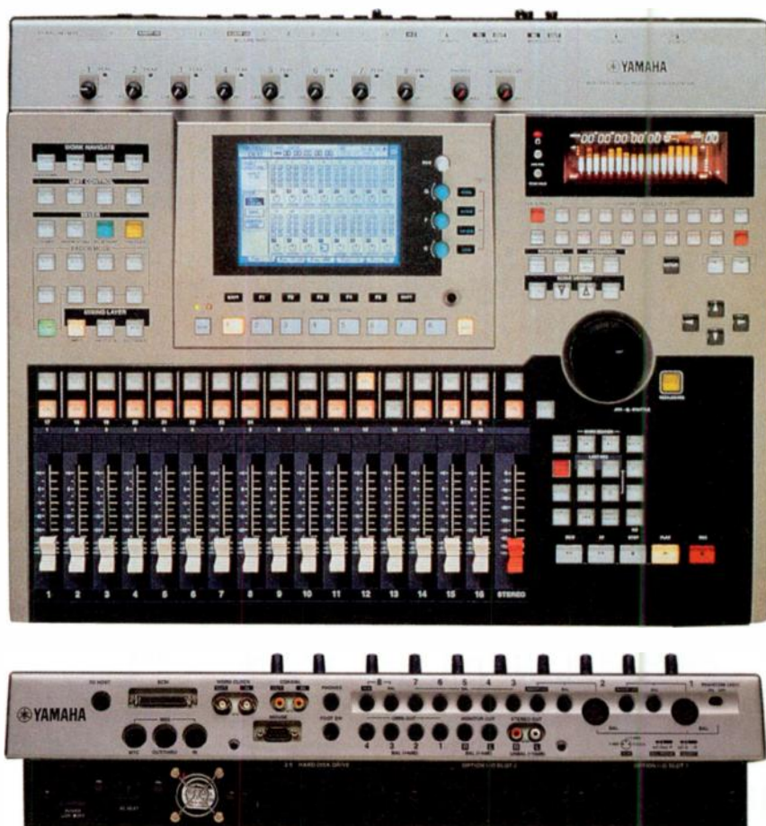
FIG. 7: Yamaha's AW4416 is the only unit that features a large dedicated meter display. That is a welcome feature if you need to monitor your levels from a distance.
