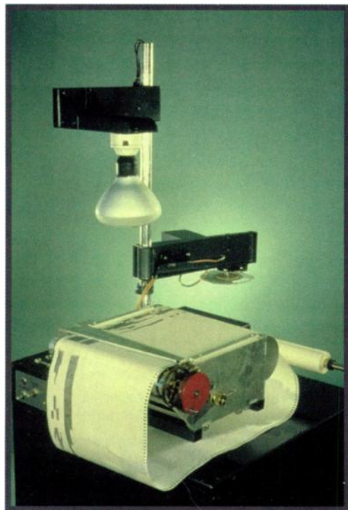
FIG. 7: The Spectrogram (1966) could control instruments' volume levels, such as Oscillator Banks or the Multi-track. Light-sensitive controllers read the markings on the chart paper.
