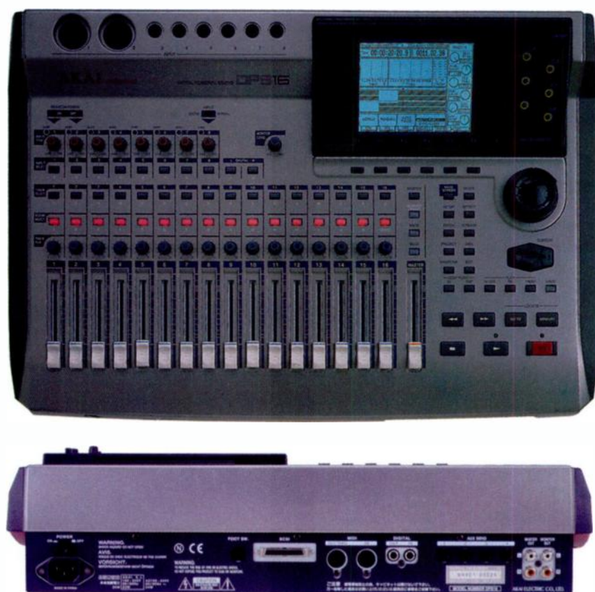
FIG. 3: The Q-Link knobs found at the upper right of the Akai DPS16 screen let you make real-time changes to channel EQ or effects settings.
