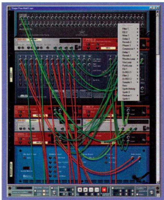
FIG. 2: Audio and CV routings are made on the rear of the rack. Shown is the back of the rack in Fig. 1. The menu in the inset at top right appears when you click on an input jack.
