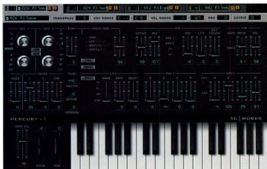
FIG. 1: On Mercury-1's front panel, four Voice Tabs across the top let you select the active voice for programming and playing with the onscreen keyboard. If you're using Steinberg's Cubase VST, the sliders, buttons, and knobs can be automated on playback.
