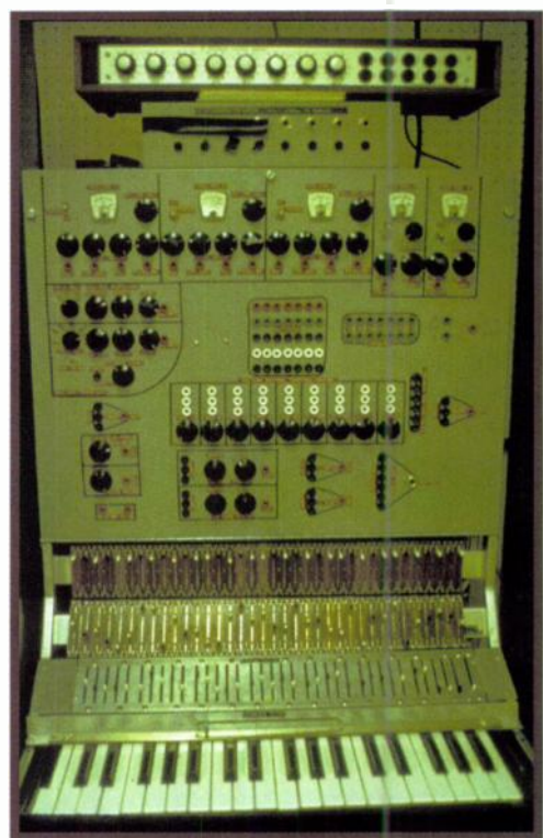
FIG. 10: The Polyphone (1970) had an extensive control panel. Each key had waveform and pitch controls.
