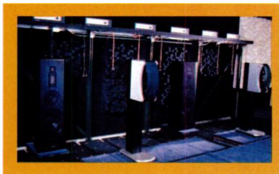
FIG. 1: Speakers mounted on pneumatic platforms can be shuffled to prevent listeners from becoming acclimated to their positions.
