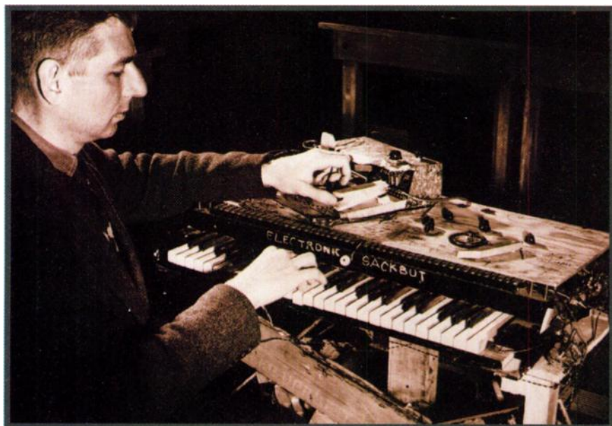
FIG. 1: When Hugh Le Caine played the 1948 prototype of the electronic Sackbut, his right hand controlled the touch-sensitive keyboard while his left hand controlled timbre.
