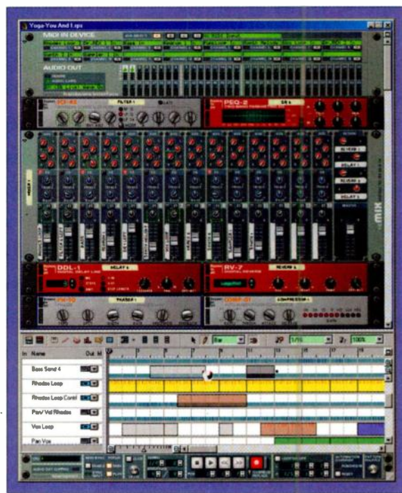
FIG. 1: Reason's visual interface is a scrolling rack of modular gear. The Hardware Interface at the top and the sequencer at the bottom are staples. Modules occupy differing amounts of space in the rack, but individual modules cannot be resized. You can minimize a module by clicking on the small gray triangle in its upper-left-hand corner.
