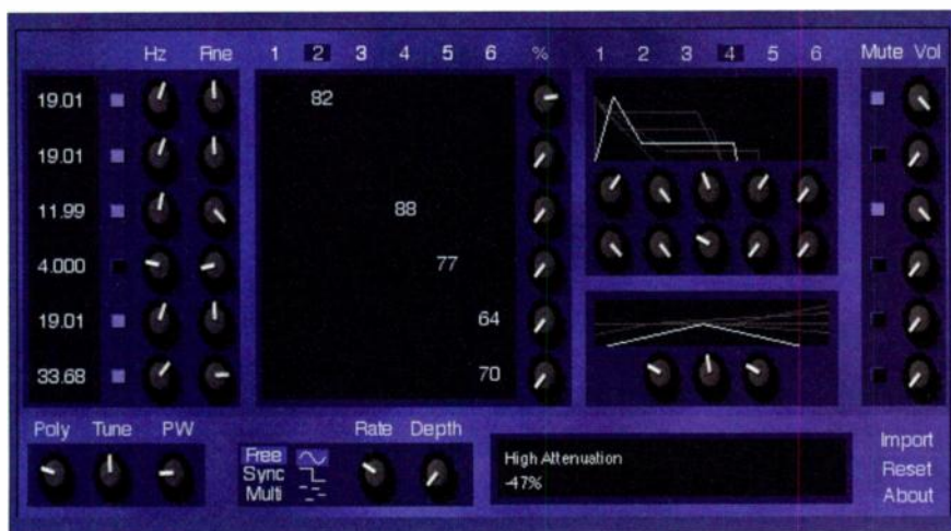
FIG. 1: FMHeaven is the latest and most sophisticated of the Ces soft synths. It features a 6-by-6 modulation matrix that lets an oscillator modulate any other and can also load Yamaha DX-7 patch banks.
