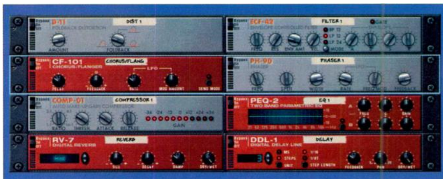
FIG. 6: Reason includes a variety of standard half-rack effects that can be patched in-line between modules and the mixer or used as send destinations.
