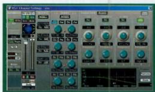
FIG. 3: Channel Settings can be displayed for each VST Mixer channel. In addition to duplicating the selected channel strip, the window affords access to four inserts, eight effects sends, and four EQ modules with an EQ curve display.
