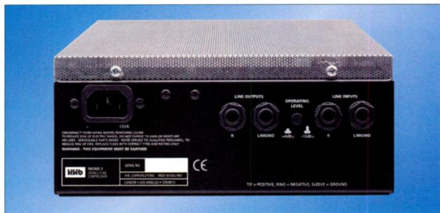
FIG. 1: The Fat Man's rear panel provides balanced/unbalanced 1/4-inch inputs and outputs. The operating level is switchable between +4 and -10 dBu.
