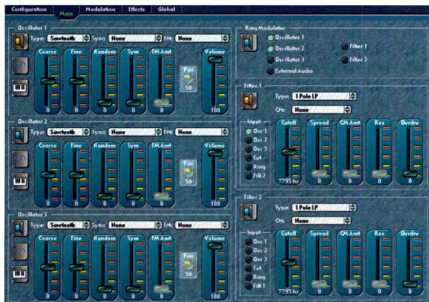
FIG. 3: Retro 's Program Editor's Main page is where oscillator, audio-rate modulation, and filter settings are made. The signal path can also be controlled from this page with the Speaker and Input buttons.
