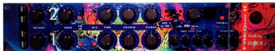
The Freque II from the United Kingdom's DACS is a dual ring-modulator boasting CV inputs, frequency shifting, and FM capabilities.
