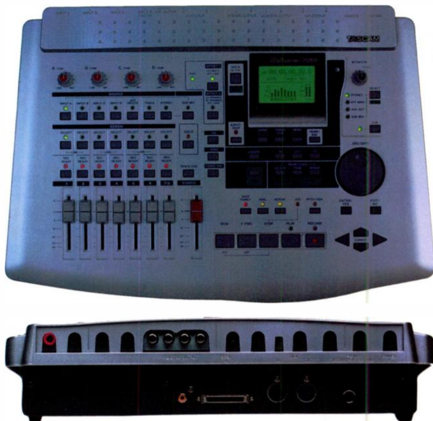
FIG. 4: The Tascam 788 packs 250 virtual tracks into a very small footprint. Virtual tracks can be allocated to any physical tracks.
