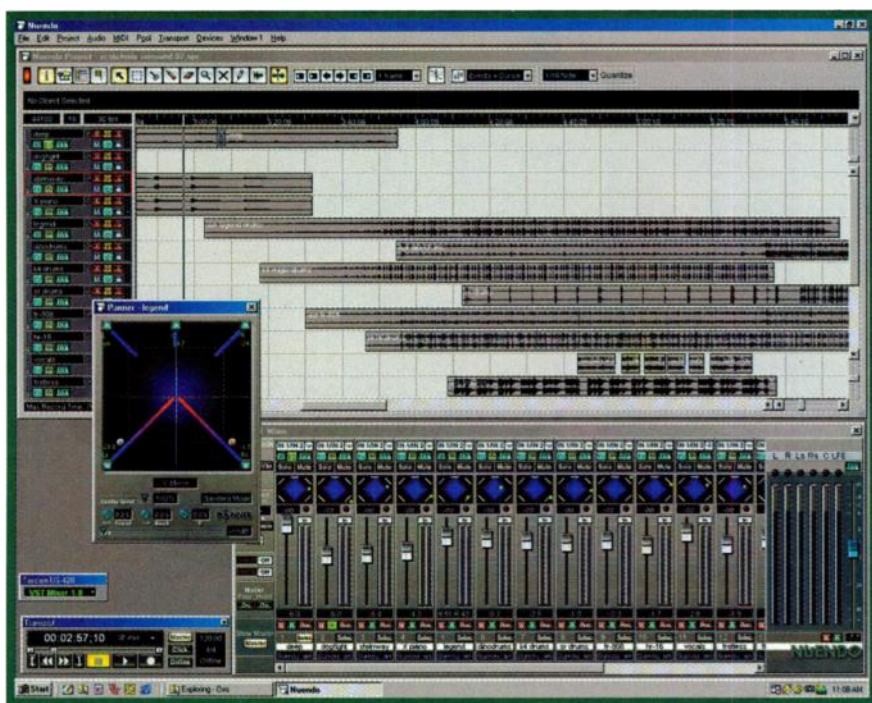
FIG. 1: Nuendo is a complete software-based workstation for audio post, interactive media, and music production. Its tools provide recording, editing, processing, and mixing in mono, stereo, and eight channels of surround sound in a variety of formats.
