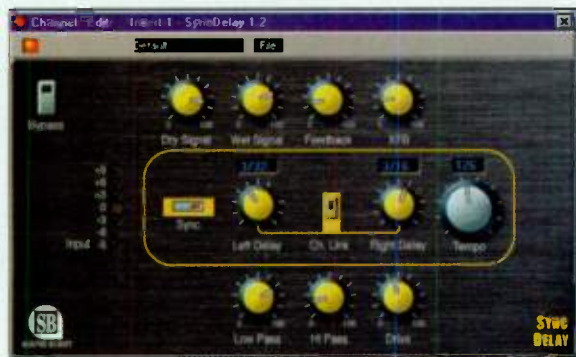
FIG. 1: The Sync Delay plug-in can synchronize its output channels to a specified tempo. The independently adjustable left and right output channels can also sync to each other.
