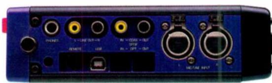
FIG. 2: HHB's Portadisc includes a wealth of input and output connectors, including USB for digital-audio transfers to a laptop.
