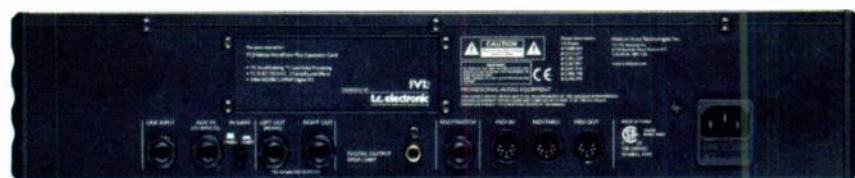
FIG. 2: VoicePrism's rear panel provides 1/4-inch TRS balanced line and auxiliary inputs and a switch to change input sensitivity from +4 dBu to -10 dBV. Also included are a pair of 1/4-inch TRS balanced analog outputs, an S/PDIF output, three MIDI ports, and a control jack that works with one- or three-button footswitches. An expansion port accepts the optional VoiceCraft expansion card.
