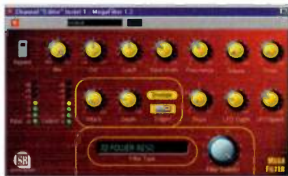
FIG. 2: Mega Filter offers ten filter types with a lot of flexibility, including five cutoff slopes.
