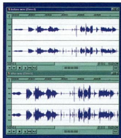
FIG. 2: The file in the lower window of Sonic Foundry's SoundForge was processed with a dynamic compressor and normalized. Note how much more signal is available than in the top window.
