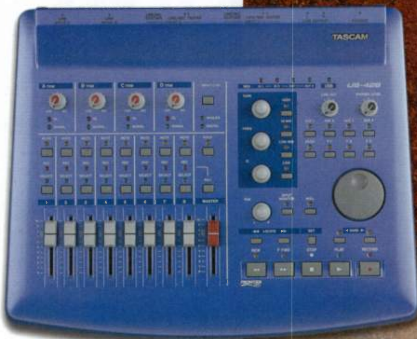
FIG. 1: The Tascam US-428 includes a full complement of faders, buttons, and knobs designed to give you tactile control over your music-software mix functions.
