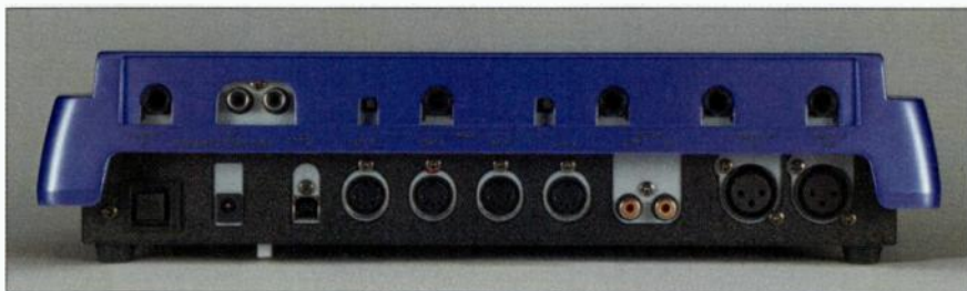
FIG. 2: The US-428's back panel features plenty of audio and MIDI connectivity, including mic-level, balanced and unbalanced line-level, and high-impedance analog inputs along with a headphone output, S/PDIF I/O, and 32 MIDI channels.
