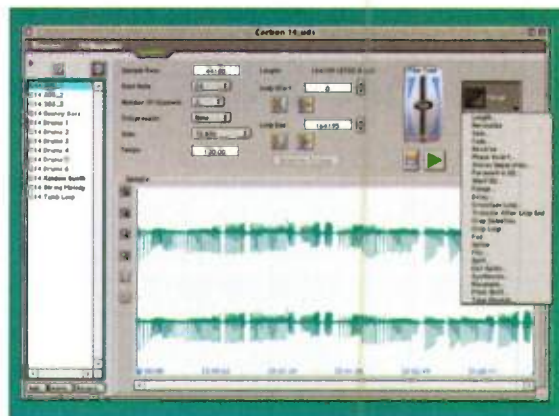
FIG. 8: Unity DS-1's Samples page provides a stereo waveform display and a complete set of sample-editing tools. If you need a tool Unity doesn't offer, link it to an external waveform editor.
