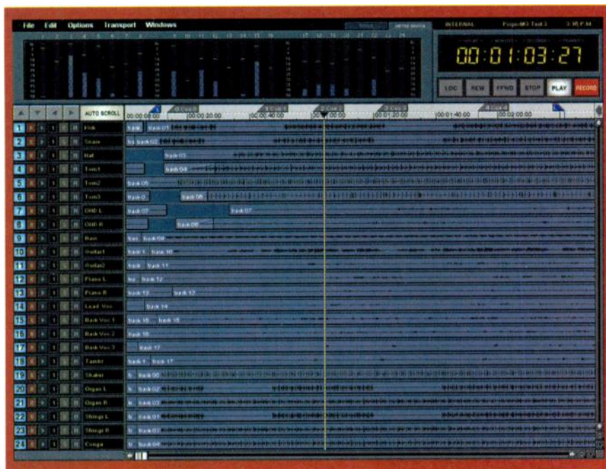
FIG. 3: The HDR24/96's GUI software gives you DAW-like editing capabilities in addition to extra recording functionality not available from the front panel.
