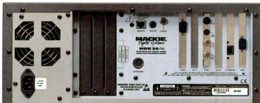
FIG. 2: The rear panel has slots for three 8-channel audio cards, so you can mix and match analog, AES/EBU, TDIF, and Lightpipe I/O.
