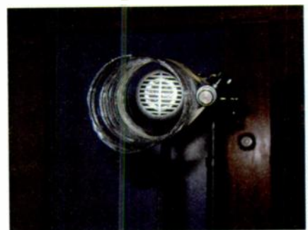
FIG. 2: You can create strange resonances by shrouding vocal mics with tubular items. A water bottle positioned around a Green Bullet produces a truly tweaked tone.
