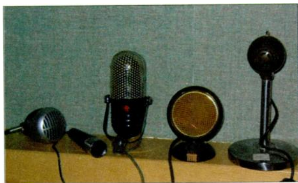
FIG. 1: The author's collection of mics for capturing off-kilter sounds includes (from left) a Shure 520D Green Bullet; a generic cassette-recorder mic; a cheap knockoff designed to look like an RCA 77; and two yard-sale gems, origins unknown.
