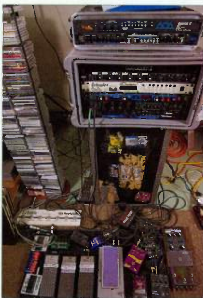
Torn's sound originates with this specially designed looping rig, which includes a modified Lexicon PCM 42 and an assortment of effects pedals and processors.
