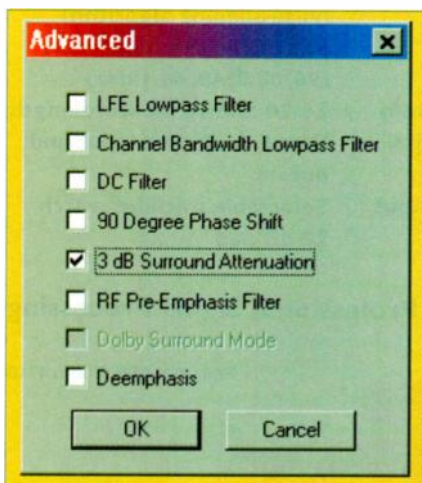
FIG. 4: SurCode Dolby Digital's Advanced screen lets you attenuate the rear surround channels by 3 dB, in addition to offering other advanced features.
