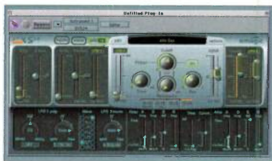
FIG. 1: Reminiscent of a synthesizer's front panel, EXS24 's Editor view provides access to two ADSR generators, two LFOs, and a versatile lowpass filter.
