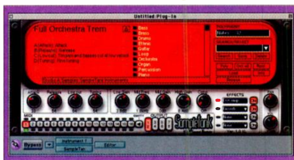
FIG. 6: SampleTank is a VST Instrument that provides all the basics needed for sample playback. Its knobs change identities depending on which instrument and effects you select.
