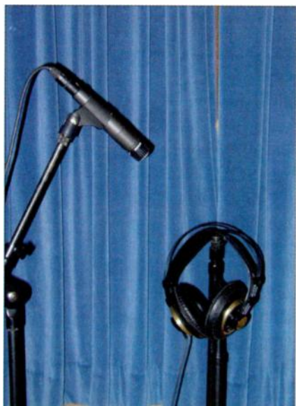
FIG. 3: A great way to capture small yet highly intelligible vocals is to mic the signal being played through headphones.
