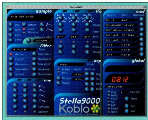
FIG. 7: Stella9000's bright-blue virtual brushed-metal panel offers an amazing filter and extensive modulation. Part of Kobo's Studio9000 suite, Stella9000 is 8-note polyphonic, but not multitimbral.
