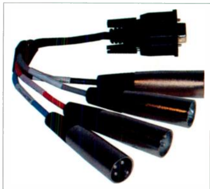
FIG. 3: The optional breakout cable attaches to the 9-pin connector on the back of the DigiMax to provide four stereo pairs (eight channels) of AES/EBU digital output. A similar cable for S/PDIF output is also available.
