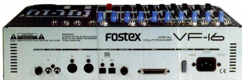
FIG. 1: Digital I/O on the Fostex VF-16 can be switched from S/PDIF to ADAT format, providing eight additional simultaneous recording inputs.
