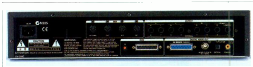
FIG. 2: The XV-5080 features word clock in and three digital outputs: coaxial S/PDIF, optical S/PDIF, and Roland R-Bus. You can configure the balanced outputs as four pairs or eight individual outs. Two MIDI Ins allow 32-channel operation, and a SCSI port connects to peripherals such as a CD-ROM or Zip drive.
