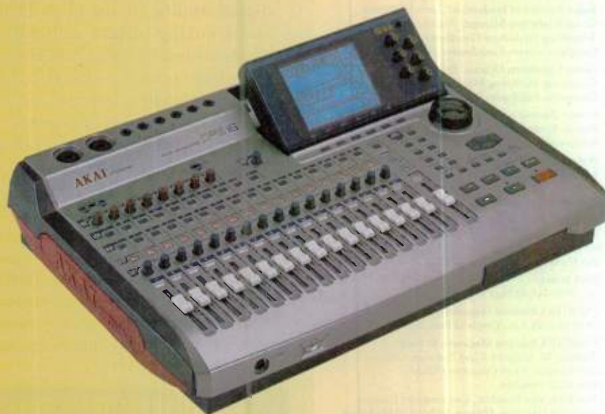
Akai's user-friendly DPS16 features Q-Link knobs in the upper right of the unit, which let you make real-time changes to channel EQ or effects settings.
