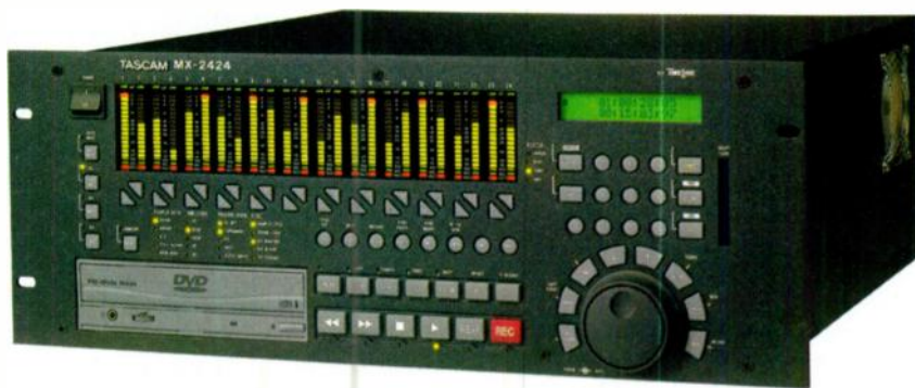
FIG. 2: The 24-track MX-2424 provides 24-bit, 96 kHz audio and a wealth of editing tools.
