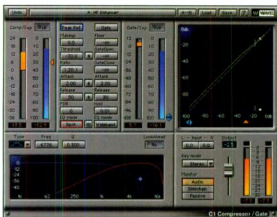
FIG. 2: C1 Compressor/Gate combines a compander with a gate/expander. The signal can be split (bottom left) into active (red) and passive (blue) zones. The active zone can be used for the main signal and the sidechain.
