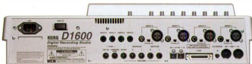
FIG. 1: The Korg D1600's rear panel boasts eight 1/4-inch balanced inputs, four XLR jacks, and S/PDIF digital I/O.
