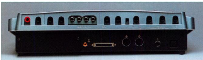
FIG. 2: The Tascam 788's rear panel provides four 1/4-inch inputs, two aux inputs, and two pairs of RCA outputs along with an S/PDIF output, a headphone jack, a footswitch connection, and a SCSI-2 port.
