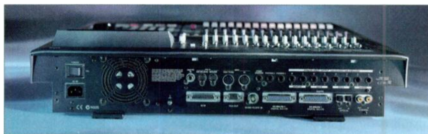
FIG. 1: The VS-2480's back panel offers mouse and keyboard inputs, a direct out for a VGA monitor, 16 microphone inputs, and two R-BUS ports.
