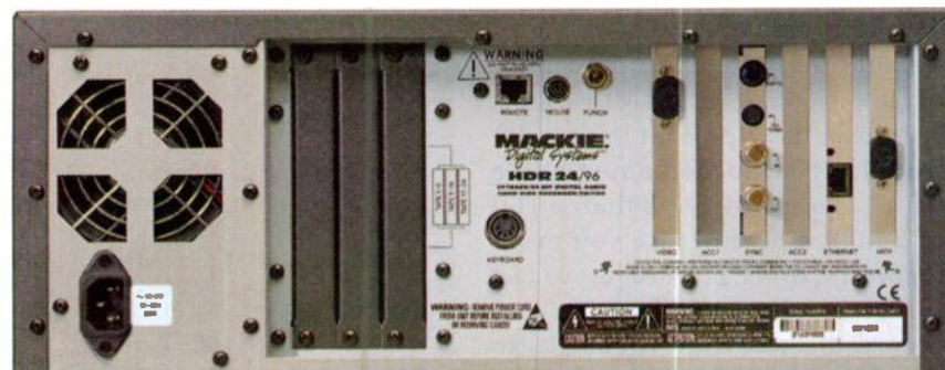
FIG. 2: The rear panel of the Mackie HDR24/96 provides a 100Base-T Ethernet port, an SVGA monitor port, and a port for a keyboard. Users can also connect a PS/2 mouse or trackball from the unit's rear panel.
