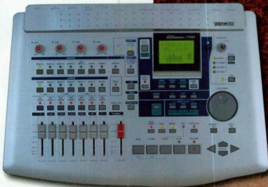
FIG. 1: The Tascam 788 Digital Portastudio sports an easy-to-use interface combined with flexible I/O options and two built-in effects processors.
