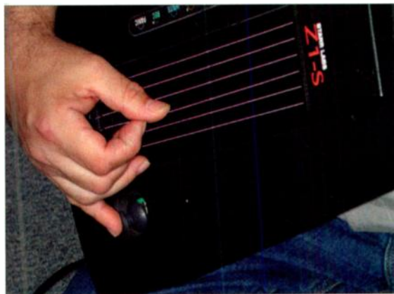
FIG. 4: The Ztar's joystick offers two modulation assignments for each axis. Depressing the joystick provides one additional controller.
