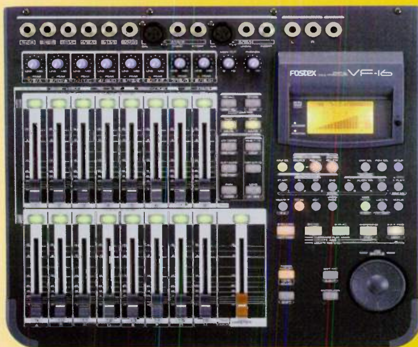
The Fostex VF-16 comes with eight channels of ADAT and two channels of S/PDIF I/O.
