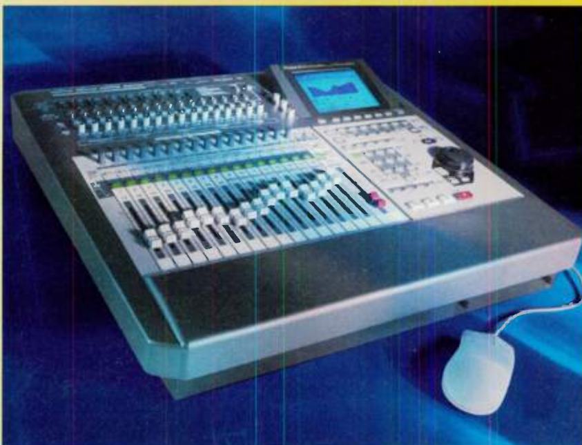
Roland's VS-2480 hard-disk recorder takes home-studio recording a step further by providing 24-track playback, mouse-based LCD editing, and the option of hooking up a VGA monitor.
