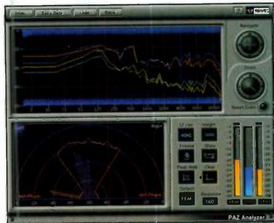
FIG. 6: The top window of the PAZ Psychoacoustic Analyzer displays the frequency spectrum with real-time (lower) and peak (upper) curves. The bottom window analyzes stereo imaging. The yellow level meters show peak channel levels, whereas the blue meter can show the peak or RMS level for the sum of both channels.
