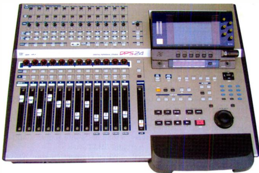
FIG. 1: The DPS24 can record 20 tracks simultaneously with 250 virtual tracks.
