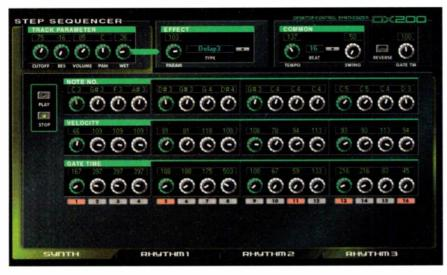
FIG. 3: The *DX200 Editor* software lets you create Patterns and Songs on your computer. The user interface resembles an analog step sequencer, with virtual knobs for note, gate time, and Velocity.
