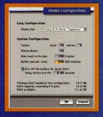
FIG. A: This dialog box in MOTU's Digital Performer lets you set the optimum buffer size and number of audio tracks to deliver the best performance for your system. The bottom of the dialog box indicates the required RAM for the current configuration.
