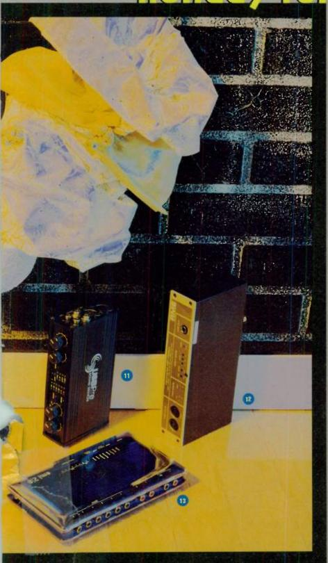
11. The Sound Devices USBPre (Mac/Win; \$695) proves that great things do come in small packages. This 2-channel device includes a pair of balanced mic preamps with phantom power and a 15 dB pad; 1/4-inch and RCA inputs; \$\$/PDIF 1/0; and a pair of headphone jacks. The USBPre uses 24-bit converters and has a frequency range of 10 Hz to 22 kHz. Sound Devices, LLC; tel. (608) \$24-0625; e-mail info@sounddevices.com; Web www.sounddevices.com.
