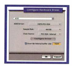
FIG. 1: MOTU's *Digital Performer* lets you easily set the sample rate and buffer size when using the ASIO driver.
