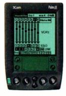
FIG. 11: Handi-Q's Handi Systems Controller Software provides a full complement of onecreen controls for several types of hardware devices.
