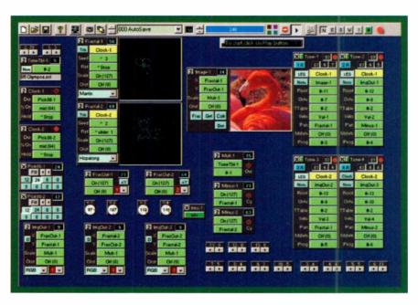
FIG. 3: SoftStep Pro can draw fractals in real time and use data extracted from the image for various control purposes. Bitmapped graphics files can also be imported and used to control other functions.
