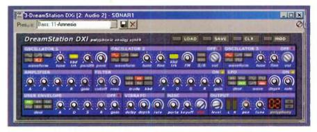
FIG. 3: Cakewalk's *Sonar* is the first program to support DirectX-based virtual instruments. DX Instruments (and VST Instruments) allow easier setup and better performance by integrating software synthesizers, such as Audio Simulation's *DreamStation DXi*, into the host program.
