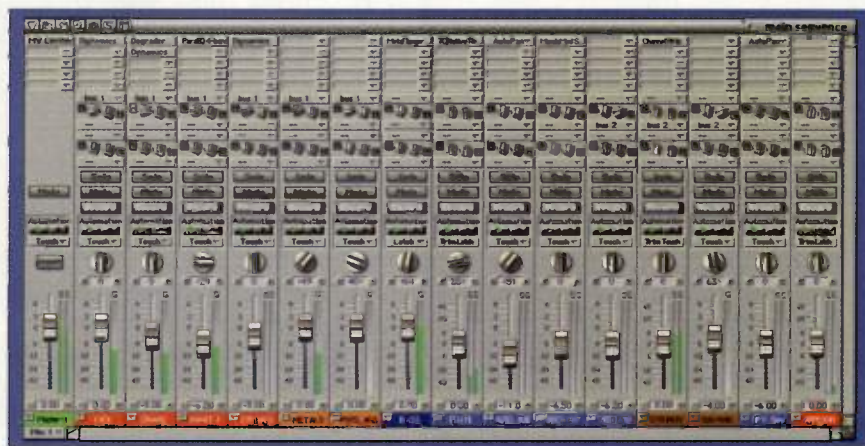
FIG. 5: The Mixer window is laid out like a hardware console. Simple to use, it displays both MIDI and audio tracks with faders, meters, sends, and Inserts for plug-ins.
