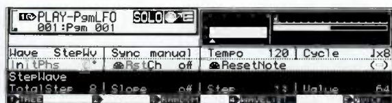
FIG. 3: The programmable StepWave LFO can feature up to 16 steps per cycle. Applied to oscillator pitch, it functions as a 16-step sequencer.
