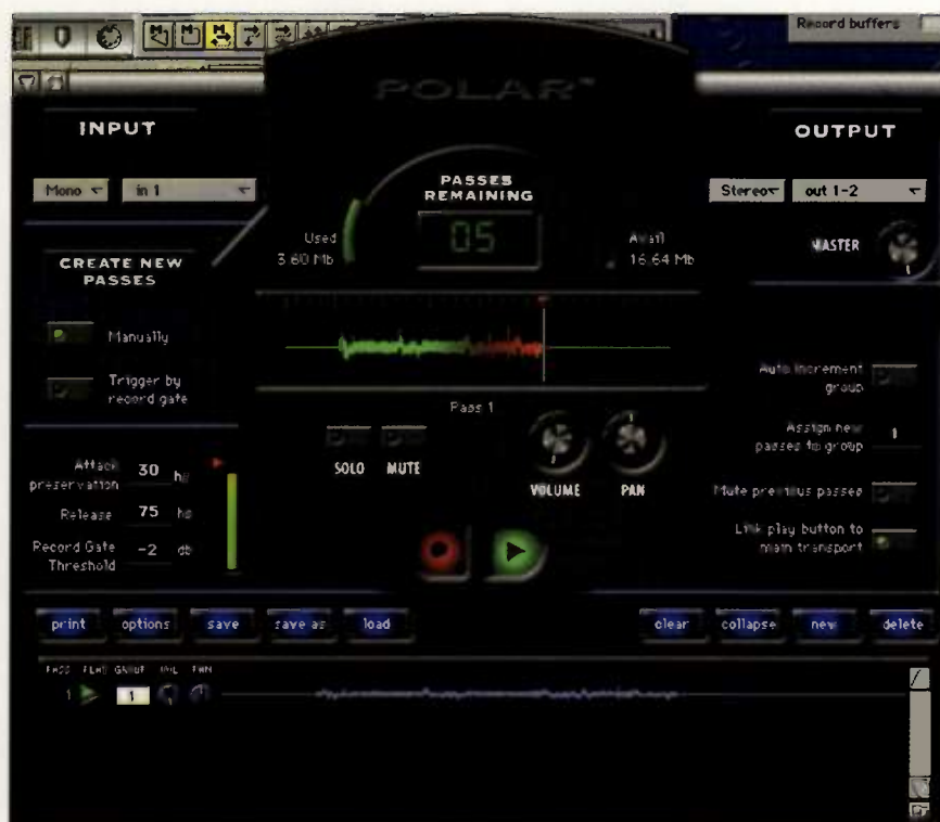
FIG. 4: The Polar plug-in's intuitive audio-recorder window is ideal for quickly recording multiple passes. You can create new takes on each pass or merge takes in real time, with the results easily imported into Digital Performer .
