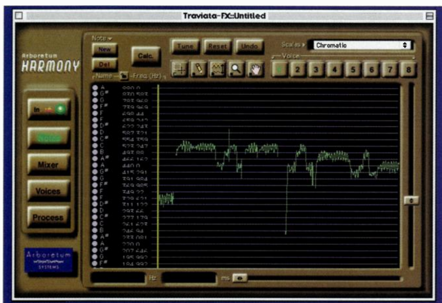
FIG. 1: Harmony 's Notes window shows the pitch curve of the currently loaded sound file. Files can conform to numerous scales, which you choose from the Scales pop-up menu in the upper right of the screen.
