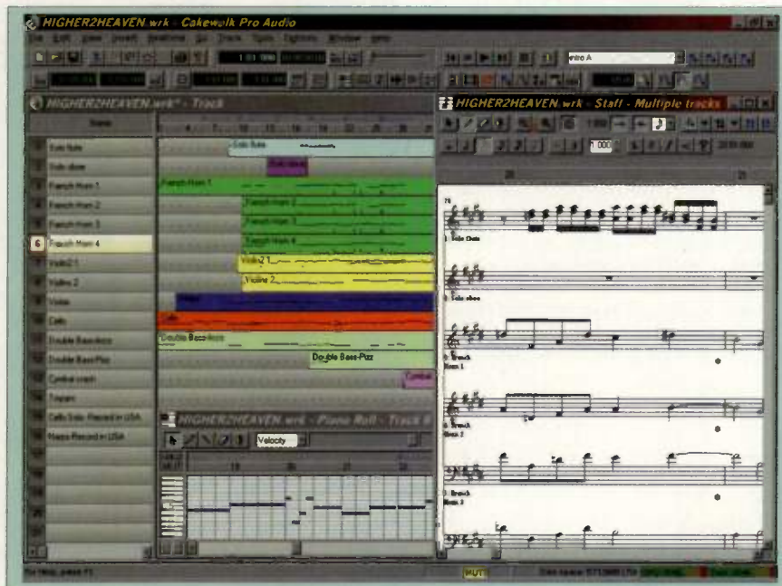
FIG. 2: This screenshot from Cakewalk's Pro Audio shows the different instrumental parts in track view and in standard notation.
