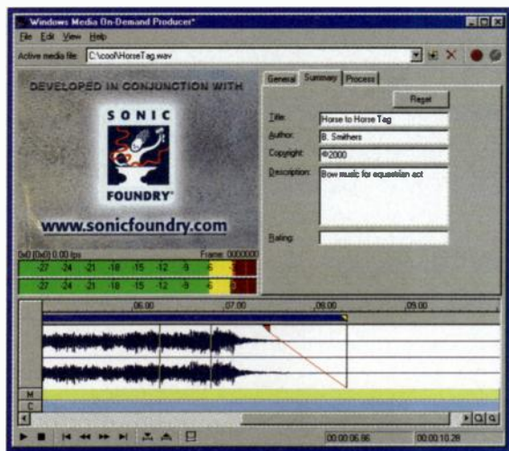
FIG. 2: Windows Media On-Demand Producer is a free utility from Microsoft and Sonic Foundry for encoding audio and video files in the Windows Media format. Audio files can be trimmed by dragging the yellow markers, and fades of varying lengths can be added by dragging the red markers.
