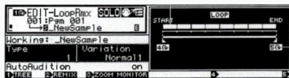
FIG. 4: The Loop Remix feature divides loops into segments and randomly reorders them. You can also save successful remix algorithms for later use.
