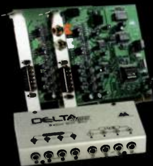
DELTA 66 & DELTA 44 - 24 bit/ 96 kHz full-duplex recording interfaces.
