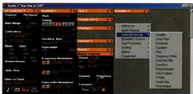
FIG. 2: The VAZ Modular interface avoids clutter by allowing you to "roll-up" each module so that only its name appears. It also uses an efficient menu system for picking the various modules you'll use in your synth designs.
