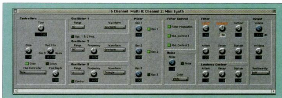
FIG. 5: The Control Panel for the Mini Synth patch will bring a nostalgic tear to many an eye. Parameters displayed in red (filter Cutoff and Emphasis) have MIDI modulation controllers assigned to them.
