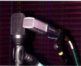
FIG. 1: One helpful trick is to set up two different mics side by side and record the harmonica simultaneously to two tracks. That not only fattens the sound but also allows for "organic" equalization—the two tracks can simply be blended to taste during mixdown—alleviating any need for EQ. Shown are two of the author's favorite mics for recording harmonica: the Microtech Gefell MT 711S condenser and Sennheiser 441 dynamic.
