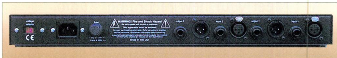
FIG. 2: The HM-1's rear panel provides XLR and 1/4-inch inputs and outputs. The 1/4-inch input jacks can handle high-impedance mic signals.
