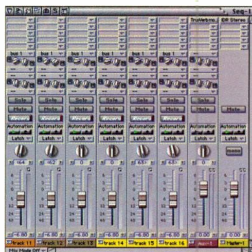
FIG. 4: You can lessen the strain on your DAW's CPU by using an aux track to apply a plug-in to several tracks at once. Here, an aux track receiving input from bus 1 in Digital Performer receives effects-send signals from several tracks. The aux track then sends those combined signals to a Waves reverb plug-in by way of the aux track's insert.
