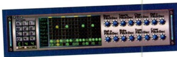
FIG. 3: Psion is one of four identical Storm drum boxes. Each drum box has its own set of eight classic sampled drum sounds. Psion's samples are from the Roland TR-808 and TR-909.
