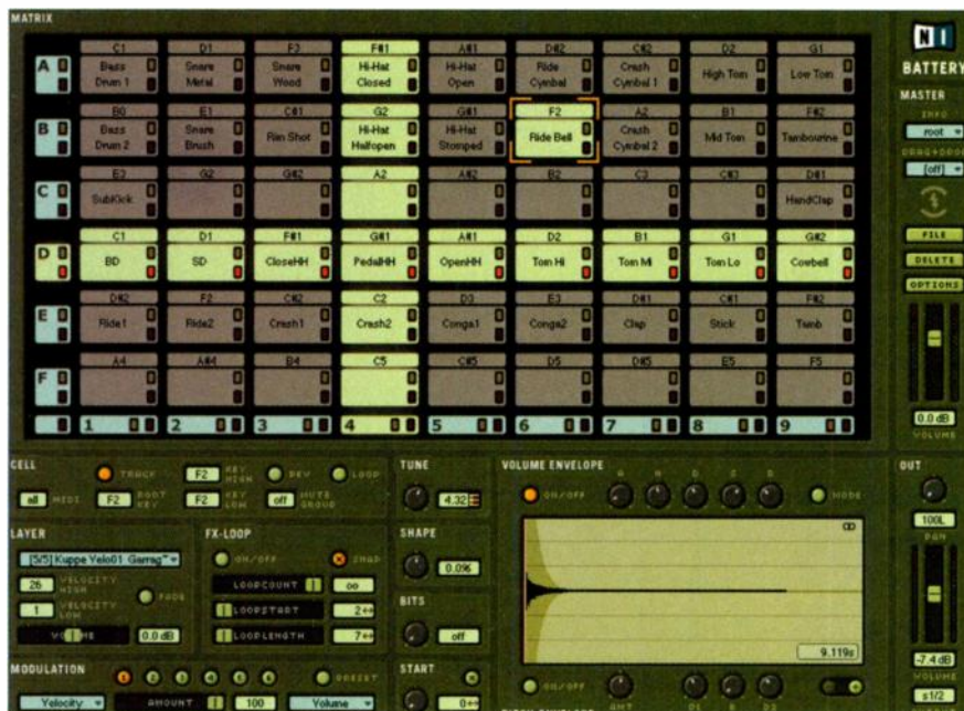
FIG. 1: Battery 's control panel features 54 drum pads (Cells) arranged in a six-by-nine Matrix. Six control sections below the Cell Matrix provide extensive real-time manipulation of sample playback.
