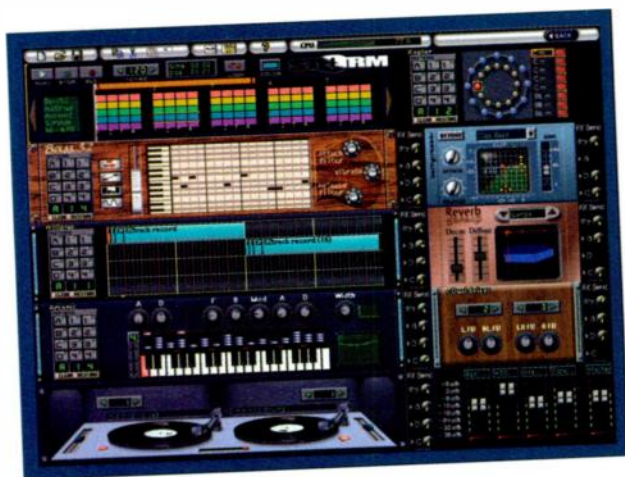
FIG. 2: Storm 's Composer is a colorful collection of the instruments, effects, and other modules in your Rack. Most instruments have 16th-note Pattern Sequencers for programming one-measure loops. The Song Sequencer at the top automates pattern and front-panel control changes.
