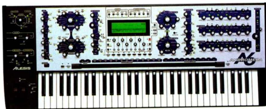
FIG. 1: One of the few polyphonic analog synthesizers in production, the Andromeda A6 offers a wealth of knobs and buttons for extensive hands-on control. Every control transmits MIDI data and every parameter responds to MIDI data, so that you can automate every real-time edit recorded into a sequencing program.
