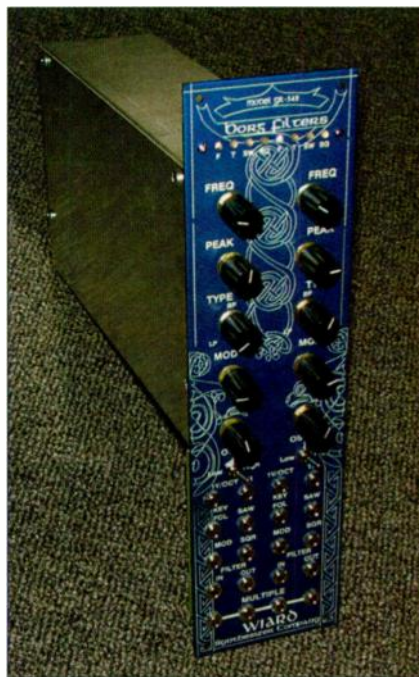
FIG. 3: Based on the Buchla Lopass Gate and the Korg MS-20 filter, Wiard's Borg Filter offers two independent Vactrol-based filters with individual VCOs.
