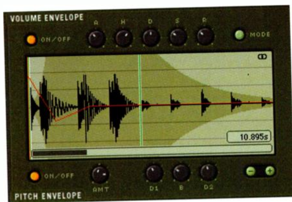
FIG. 2: Battery's Envelope and Wave Display section shows the Volume Envelope (green shading), the Pitch Envelope (red line), and the user-defined FX-Loop (left of the green vertical line) for the selected Cell.
