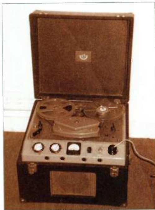
FIG. 1: This EMI TR51 was Meek's primary mixdown machine until early 1963. It had three heads, took reels as wide as 8.25 inches, and ran at 15.0 and 7.5 ips.
