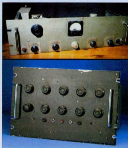
FIG. B: These are two of Meek's so-called black boxes: the Langevin-based compressor/limiter (top) and the Pultec-based equalizer (bottom).
