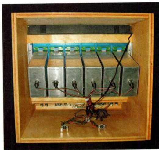
FIG. 2: The electronics for each module are housed inside an aluminum enclosure. Notice that each 5-pin DIN jack powers three modules.
