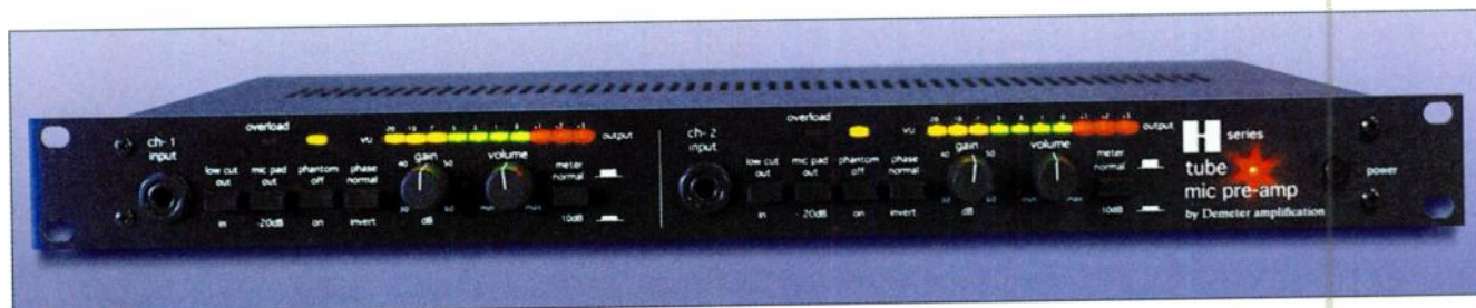
FIG. 1: Designed for the personal-studio market, Demeter's HM-1 (soon to be HXM-1) tube mic preamp likely will also win fans in higher places, thanks to its quality build and superlative sound. The unit employs a hybrid tube/solid-state circuit design.
