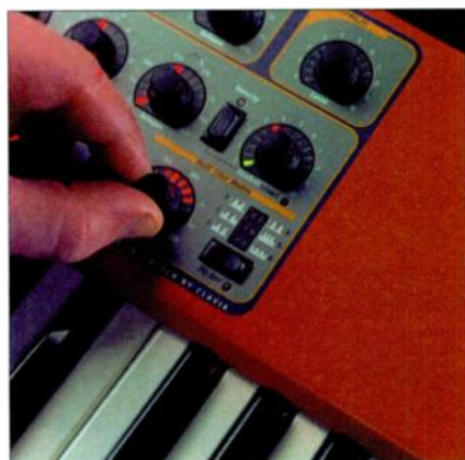
FIG. 2: The Nord Lead 3 uses digital knobs to adjust parameter settings. LEDs indicate the position of the knob, which makes editing easy.
