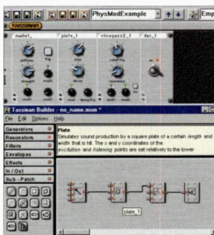
FIG. 3: Applied Acoustics' Tassman is a modular virtual synthesizer built on physical-modeling principles. The Player view (top) and Builder view each show the primary building blocks of a PM synth. Impedance effects are built into the plate and controlled by the Decay knob. Each module features modulation inputs, and various other parameters can be controlled by MIDI.
