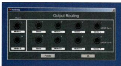
FIG. 3: Each Q10 output can carry any of the available audio signals. From the Routing screen, you can choose from sources that include any playback channel, any input channel, a mix bus, a test tone, or digital silence.
