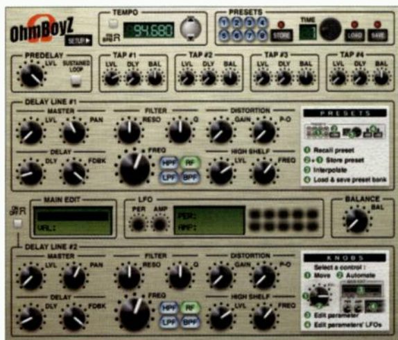
FIG. 1: OhmBoyz's processing begins with a four-tap Predelay section, followed by parallel delay lines with multimode filters and distortion. Most controls have dedicated LFOs. The Classic-style control panel is shown.
