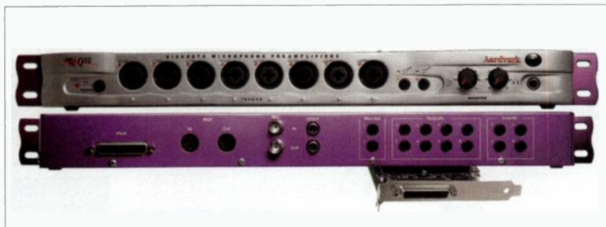
FIG. 1: The Q10 computer audio interface lets you record and play back ten channels without a mixer. Eight combo jacks with mic preamps are located on the front panel. On the back panel are ports for the host PCI card connector, MIDI I/O, word-clock I/O, S/PDIF I/O, four effects inserts, stereo monitor outputs, and eight analog audio outputs.
