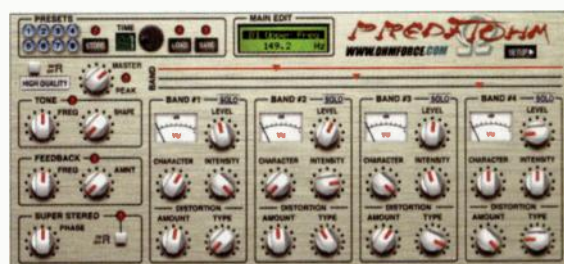
FIG. 2: As many as four user-definable bands of compression or expansion are available in the Predatohm multiband compander. Each band also offers 13 types of distortion. The Classic-style control panel is shown.
