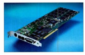
FIG. 3: Audio interfaces with digital signal processing (DSP) chips, such as this Korg OASYS PCI, can often apply effects to incoming audio. That allows you to hear effects while recording—without the latency you would get if the signals were processed on the computer itself.
