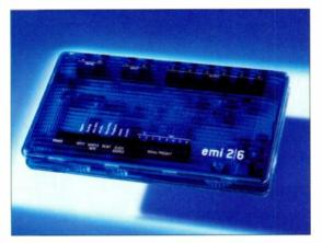
FIG. 2: A growing number of computer audio interfaces, such as the Emagic EMI 2/6, offer zero-latency monitoring. By routing incoming audio directly to the interface's output rather than looping it through the computer, this design allows you to hear yourself with no delay as you record.
