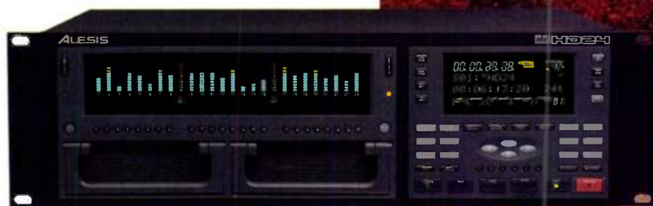
FIG. 1: The 24-channel Alesis ADAT HD24 modular hard-disk recorder promises to breathe new life into the ADAT series. The stock unit supports a word depth of 24 bits and sampling rates as high as 48 kHz, but you can record at a rate as high as 96 kHz with an optional I/O board.
