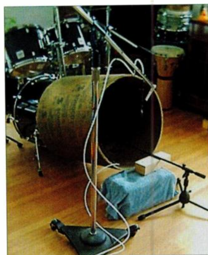
FIG. 5: When recording kick, the author often uses a Sonotube to construct a tunnel around the drum. A close dynamic mic grabs the attack while at the tube's end, a large-diaphragm condenser (shown is a Microtech Gefell M71KMT) captures enhanced resonance.
