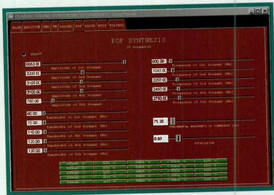
FIG. 3: Luca Pavan's Classic Sound Synthesis Techniques instrument is an elaborate interface that incorporates several synthesis methods, a waveform generator, a granular synthesizer, and four filters. The instrument runs under DirectCsound and is easy to use, but customizing it requires some knowledge of Csound.
