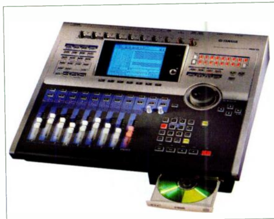
Yamaha's AW2816 offers 16 tracks of 24-bit, 48 kHz audio and provides a number of options for analog and digital I/O.
