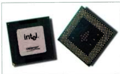
FIG. 1: Intel's Celeron processor is popular among overclockers for the relatively high degree to which it can be accelerated.
