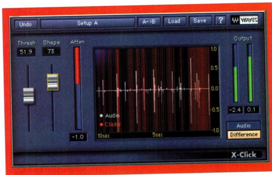
FIG. 1: Clicks and pops in vinyl recordings (and other sources) can be removed with X-Click. Detected clicks are shown in red. In some severe cases, using milder settings and processing the audio twice produces better results. In this example, the clicks being removed from the audio are monitored by switching the Difference button on.
