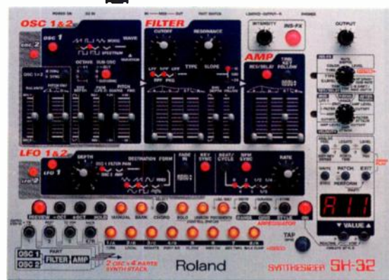
FIG. 9: The Roland SH-32 is a tabletop synthesizer with independent synthesis and percussion channels and a sophisticated arpeggiator.
