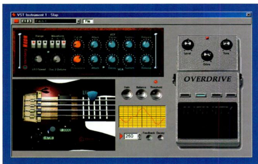
FIG. 4: This layered-bass VST Instrument was created in Infinity from within Cubase. The instrument was configured by combining two other VST Instruments, Neon and VB-1, with a feedback delay and a distortion stompbox created in Infinity.
