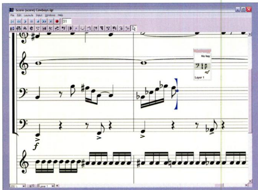
FIG. 3: In Input mode, the blue caret (cursor) indicates the current note entry position while the small Music Entry window indicates the current pitch, duration, and other parameters.
