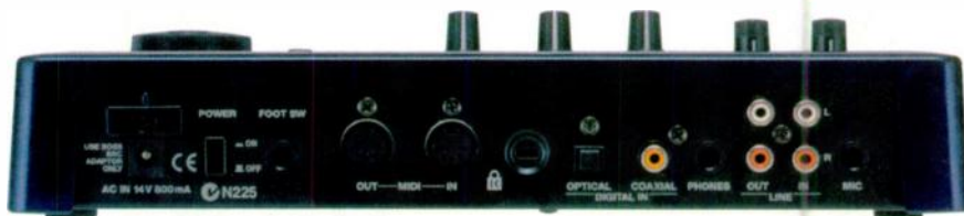
FIG. 2: Microphone, stereo line-level, and two types of S/PDIF jacks await your input. The padlock slot accepts a computer-style antitheft cable.
