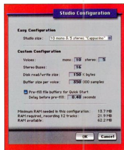
FIG. 5: The Studio Configuration dialog box lets you optimize hard-drive performance by setting the buffer size per voice.
