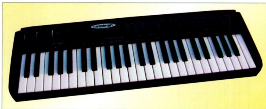
FIG. 4: Although bulkier, the Midiman Keystation 49 is functionally similar to the Edirol PC-300, but it offers a better display, an additional MIDI Out jack, and wheels instead of a paddle for Pitch Bend and Modulation.
