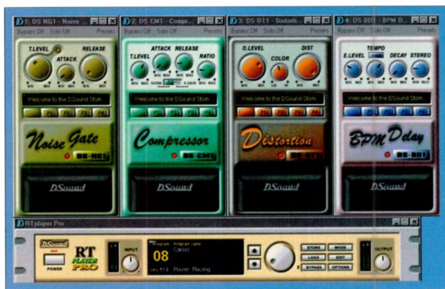
FIG. 2: DSound's RT Player Pro can turn computers into real-time multi-effects processors using VST plug-ins. The program also lets users play VST synths and samplers as real-time standalone instruments that don't require sequencer-oriented VST hosts.
