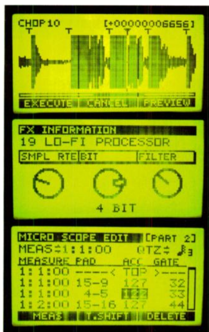
FIG. 3: The SP-505 is the only phrase sampler with a full graphic display, and it makes the most of it. These screens show the Chop feature, real-time effect control, and sequencer event editing.
