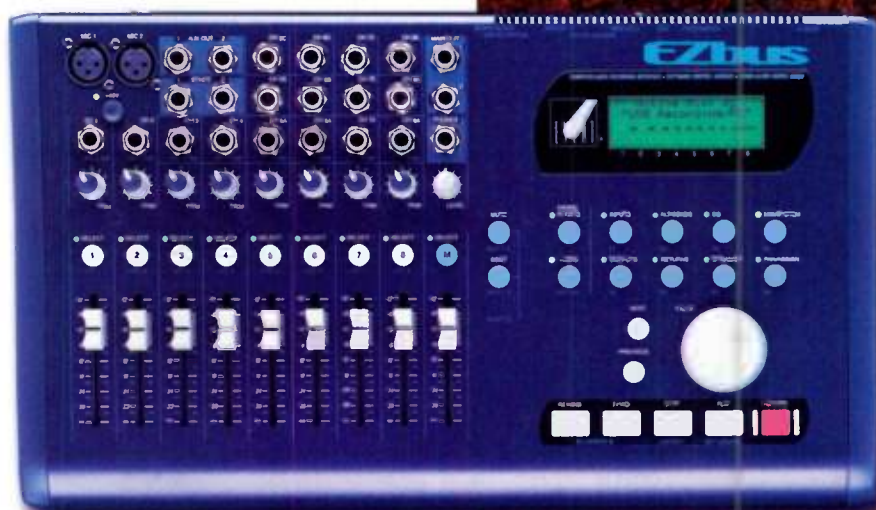
FIG. 1: The EZbus provides two mic/line inputs with phantom power, two instrument/line inputs, and four sets of three summed line inputs. In addition to the I/O functions of a digital mixer, the unit features transport and other controls for sequencing and DAW programs.
