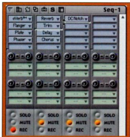
FIG. 2: Clicking the tiny box in the lower left of the insert section (as seen in the first channel) produces a double-arrowhead cursor (as seen in the third channel). You can then drag the dividing line to separate the prefader from the postfader effects. In channel two the divider appears between Trim and Delay.
