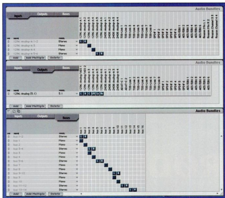
FIG. 4: The Audio Bundles window allows elaborate routing of inputs, outputs, and buses. In this composite graphic, a 5.1 surround mix is assigned discrete outputs on a MOTU 1296 audio interface. Input and output assignments are created and edited in separate displays.
