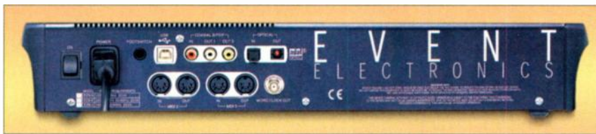
FIG. 2: The rear panel of the EZbus provides both ADAT Lightpipe and S/PDIF digital I/O (including two S/PDIF outputs), a USB port, two pairs of MIDI In and Out ports, and word-clock output on a BNC connector.
