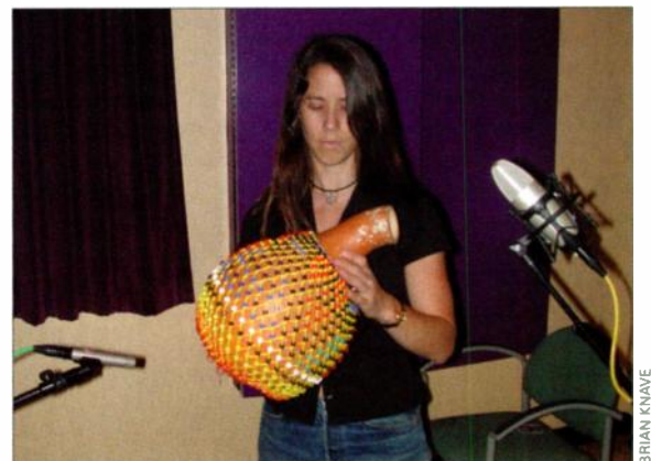
FIG. 4: Using two microphones on shekere enhances the distinction between the instrument's high and low timbres, allowing for more tonal (and spatial) control in the mix. Here, a Neumann KM 184 is positioned to pick up primarily bead slaps and finger taps and a Shure KSM32 is set up to capture the low boom coming from the mouth of the gourd.
