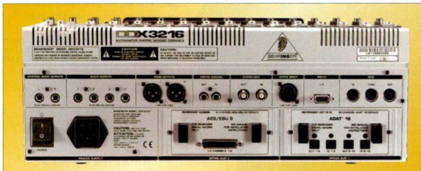
FIG. 2: In the DDX3216's rear panel, digital I/O-card slots (lower right) are fitted with the optional 8-channel AES/EBU and 16-channel ADAT cards.
