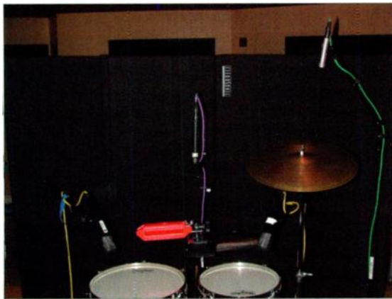
FIG. 3: This timbalito setup is miked with two dynamics and two condensers: a Sennheiser MD 421 on each drum, an Audio-Technica AT4051 over the bell/block cluster, and a Neumann KM 184 over the cymbal.
