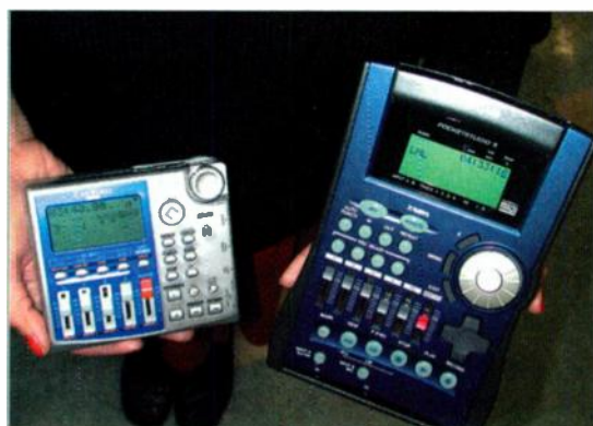
FIG. 9: The Korg ToneWorks PXR4 and Tascam Pocketstudio 5 offer the ultimate in portability. These diminutive devices record to SmartMedia and CompactFlash cards, respectively.
