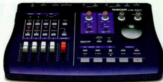
FIG. 7: The Tascam US-224 DAW controller is an example of a USB interface that is bundled with a lite version of a popular music application—in this case, Steinberg Cubasis.
