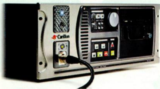
FIG. 6: A turnkey DAW puts the software you want into a rackmountable package. The Carillon system includes a fan that's quieter than most PCs.
