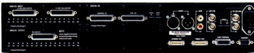
FIG. 5: A DAW interface such as Digidesign's Pro Tools 192 I/O gives you a wide variety of options for connectivity. To save space on the rear panel, DB25 connectors are used for AES/EBU, TDIF, and analog I/O.
