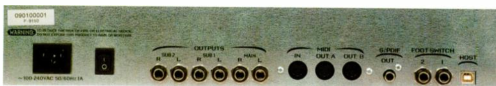
FIG. 2: The Proteus 2500's rear panel provides six analog outputs, one S/PDIF output, one MIDI In and two MIDI Out ports, two footswitch jacks, and a USB port.
