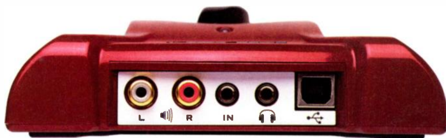
FIG. 1: The GuitarPort's rear panel provides left and right outputs on unbalanced RCA jacks, an \frac{1}{4} -inch stereo sound-card input, an \frac{1}{4} -inch stereo headphone jack, and a USB port.
