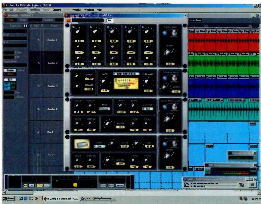
FIG. 1: The UAD-1 Powered Plug-ins can be mixed freely with native VST plug-ins in a VST host application. Here, the CS-1 channel-strip plug-in is shown running under Cubase VST/32. Performance is measured in real time using the Powered Plug-ins meter bar, shown at lower right.
