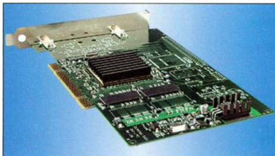
Mackie's UAD-1 Powered Plug-Ins bundle, developed by Universal Audio, includes a single-slot PCI card and a set of effects plug-ins. The card handles all processing required by the plug-ins, which takes the load off the host CPU.
