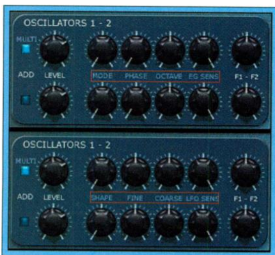
FIG. 2: Dual-function knobs such as those indicated with the red rectangles give access to more parameters without making the control panel even more crowded.
