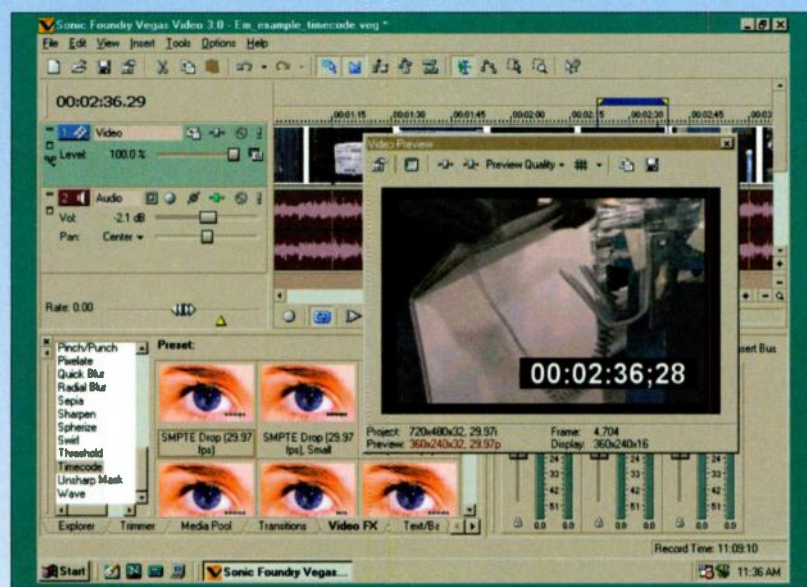
FIG. A: You can use the Timecode filter to burn a timecode window into your video.
