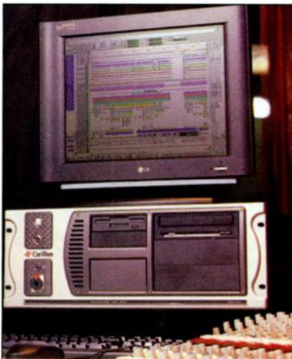
FIG. 4: Carillon Audio Systems' AC-1 computer system is especially designed for studio use. Its heavy-duty rackmount enclosure and extraquiet fans and drives keep the noise level well below that of a typical desktop computer.
