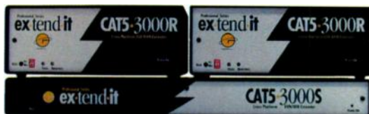
FIG. 2: Moving your computer outside of the studio into a closet or machine room requires the use of a keyboard, video, and monitor (KVM) extender such as the Ex-tend-it series from Gefen.
