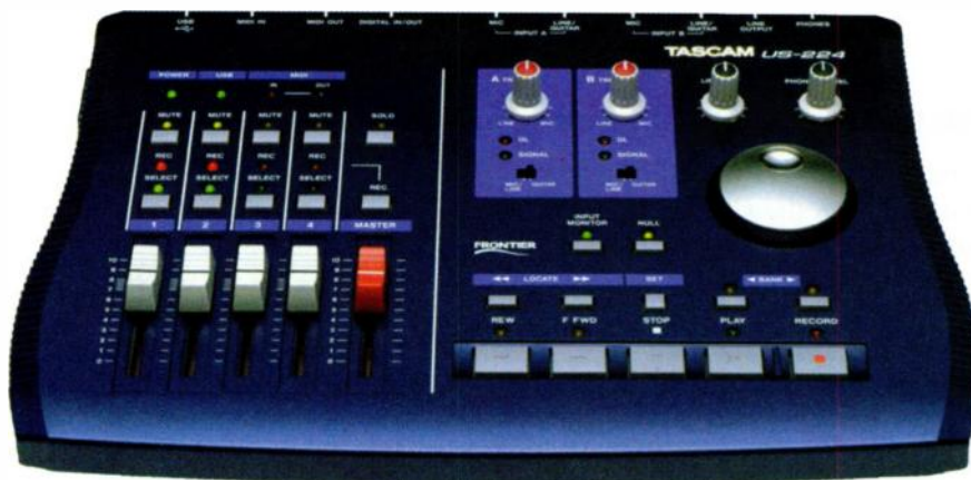
FIG. 1: The US-224 is a control surface, a 16-channel MIDI interface, and a stereo audio interface rolled into one. Bundled with a custom version of Steinberg Cubasis, the US-224 is designed to look and function like a Tascam Portastudio.
