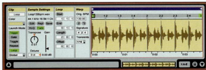
FIG. 3: The Clip view shows all the data that Live uses when it streams an audio file from your hard drive. That data is saved in a Clip file that points to the actual sound file. Each copy of a Clip file can have its own settings.
