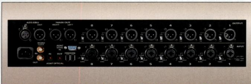
FIG. 2: The MOTU 896's rear panel is densely packed with connectors. The XLR analog audio inputs also accept 1/4-inch plugs, but the XLR outputs do not.
