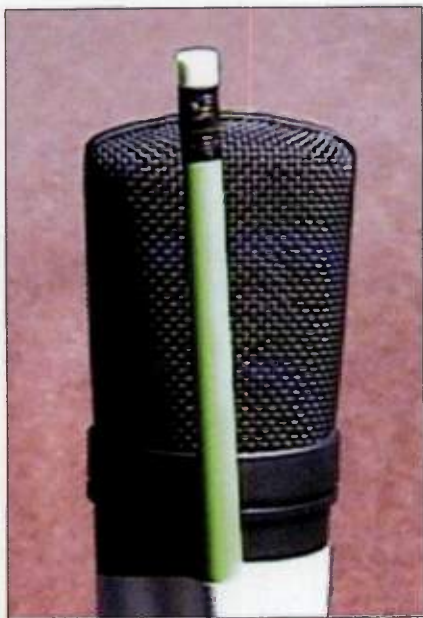
FIG. 4: One of the oldest tricks in the book for foiling plosives: simply tape a pencil over the center of the mic capsule.
