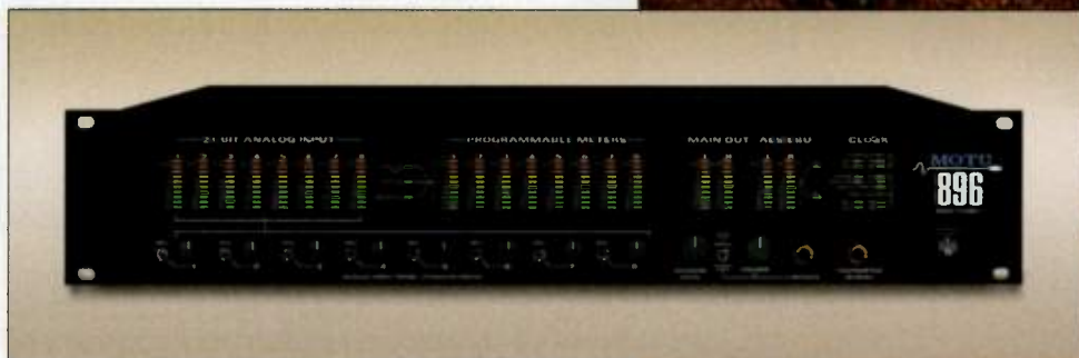
FIG. 1: On the 896's front panel are 20 ten-segment level meters with latching and continuous indication of clipping, as well as status indicators for sampling rate, digital I/O, and clock status.
