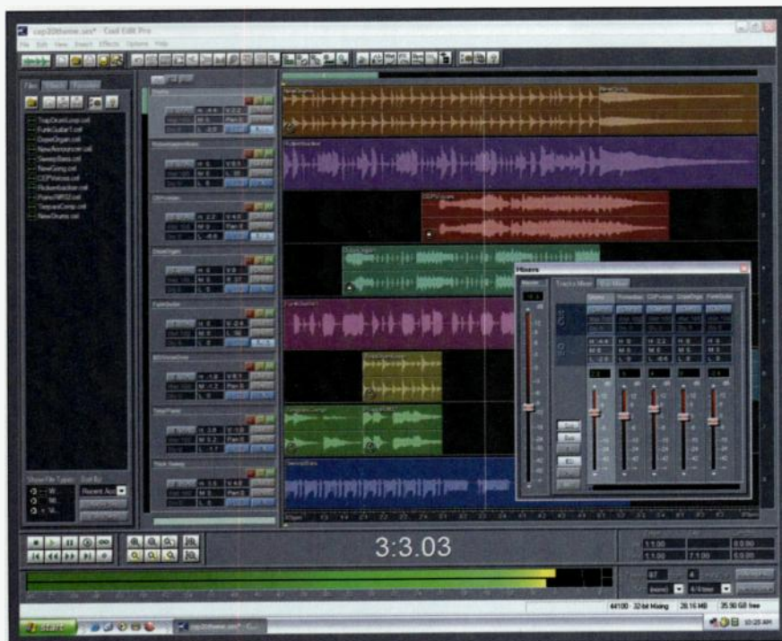
FIG. 1: Cool Edit Pro's Multitrack View supports 128 audio tracks and extensive real-time effects. The new Organizer section on the left provides easy access to files, effects, and tools.
