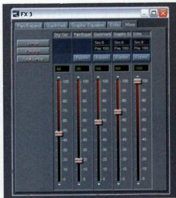
FIG. 3: Each track's Effects Rack includes an Effects Mixer where you can determine each effect's contribution to the sound of the track and configure the effects for serial or parallel operation.
