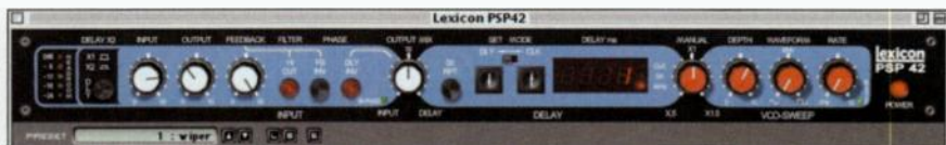
FIG. 1: The control panel of PSPaudioware.com's Lexicon PSP 42 effects plug-in is the spitting image of the original Lexicon PCM 42 digital delay processor, except for an additional knob for output-level control.
