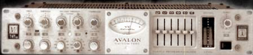
VT-747SP Stereo vacuum tube opto-compressor with LF and HF spectral side-chain control, discrete Class A six-band program equalizer and tube bypass. Excellent for stereo buss compression, audio sweetening and mastering. $2,495
