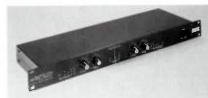
FIG. 2: The BBE 462 Sonic Maximizer is a 2-channel spectral enhancer that uses phase manipulation and filters to give your mix (or tracks) extra sparkle.
