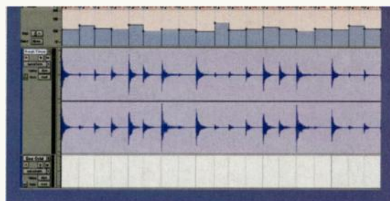
FIG. 2: This screen shot shows an example of a tempo map generated by a live percussion groove. The tempo for each 16th-note grid division can be seen next to each tempo-change marker.
