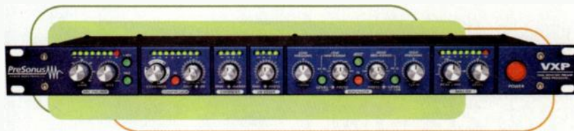
FIG. 9: Channel-strip processors combine all the essential tools for recording vocals. The PreSonus VXP includes a high-end microphone preamplifier, a dynamics processor, a de-esser, and EQ.
