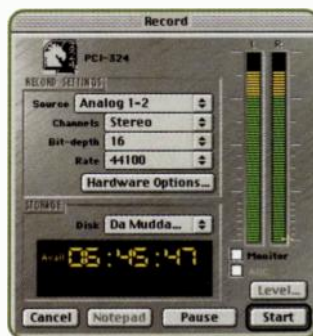
FIG. 7: When recording, set your levels so that the peaks fall just below the red zone. Record too low and you compromise resolution; go into the red and the signal distorts horribly.
