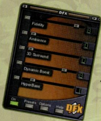
FIG. 4: Power Technology's DFX plug-in is derived from the company's high-end processors. The "Fidelity" control is an exciter; "Ambience" adds reverb.
