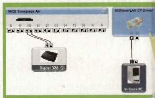
FIG. 2: In OS X's Audio MIDI Setup window, the MIDioverLAN CP Driver appears along with any attached hardware MIDI interface. Click-and-drag to make the connection between the MIDioverLAN CP driver and your external PC.
