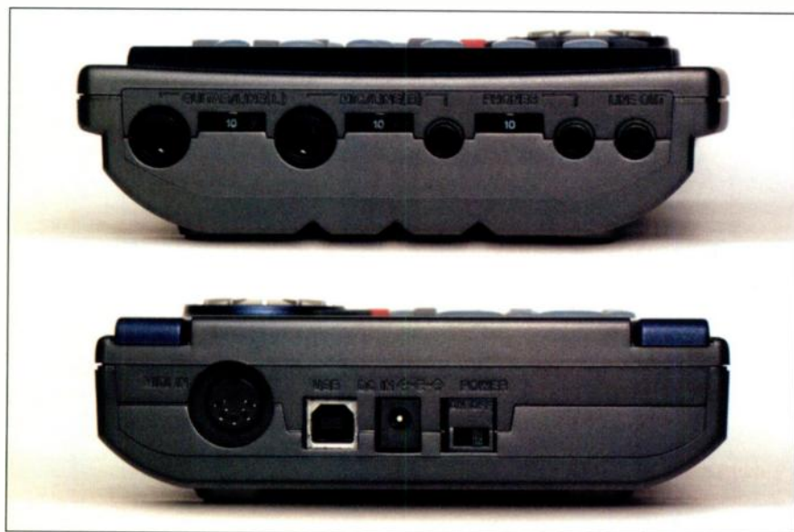
FIG. 2: Various ports are positioned on Pocketstudio 5's side panels. On the front are audio inputs and outputs. On the rear are MIDI In, USB, and AC-adaptor ports. Selector switches and the Compact Flash port are on the unit's right-side panel.
