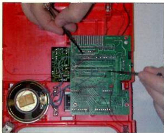
FIG. 1: For body-contact circuit bending, hold the screwdrivers in your hands as you search for places to put contacts. In this photo, switches have already been connected to the circuit board.
