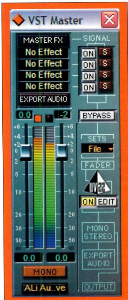
FIG. 2: Peak meters are found in analog and digital devices and generally use ladders of green, yellow, and red LEDs to indicate normal, high, and maximum levels, respectively.
