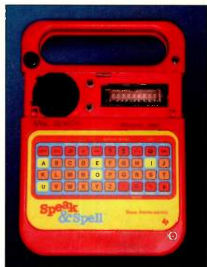
FIG. 2: This example of the Incantor, built from a Speak & Spell, has three switches (upper middle and upper right), one potentiometer (upper left), and a reset switch (lower right).
