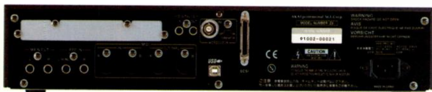
FIG. 2: The Z8's rear panel features coaxial S/PDIF I/O, a 50-pin SCSI port for external hard-drive storage, a USB connector, a BNC word-clock input, and dual MIDI I/O. Stereo analog inputs and outputs are on balanced TRS jacks.
