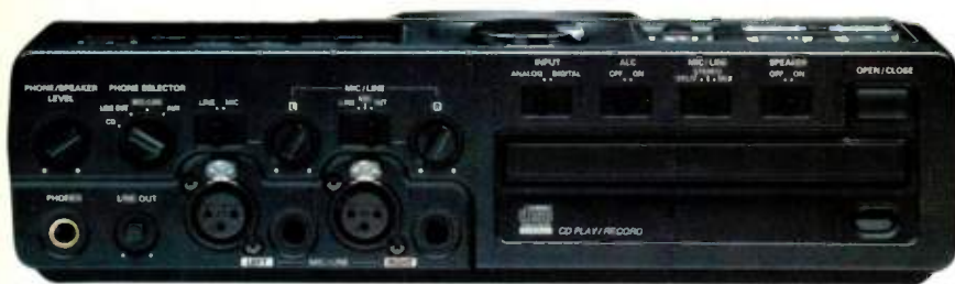
FIG. 2: Besides the CD-R drive, the front panel holds balanced XLR and 1/4-inch inputs and many of the record-related controls.
