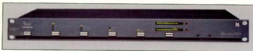
FIG. 4: The Apogee Rosetta 96's meters offer a special calibration mode that allows you to adjust the reference level to within \pm 0.1 dB tolerance.
