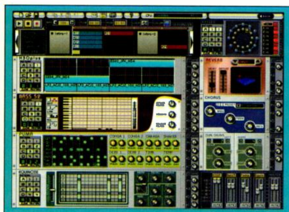
FIG. 5: Storm's rack holds four sound generators (left) and three effects processors (right). Most sound generators, including those shown, contain their own pattern sequencers at the left side of their control panels. Storm songs are constructed by recording pattern changes in the song tracks along the top.
