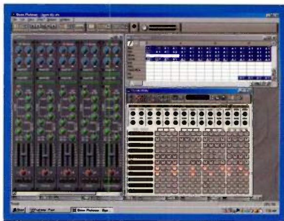
FIG. 2: Orion's control-central is its virtual mixing desk (left). All generators, such as the drum module shown here (bottom right), have dedicated pattern sequencers. Songs are constructed by selecting patterns in the song sequencer (top right).
