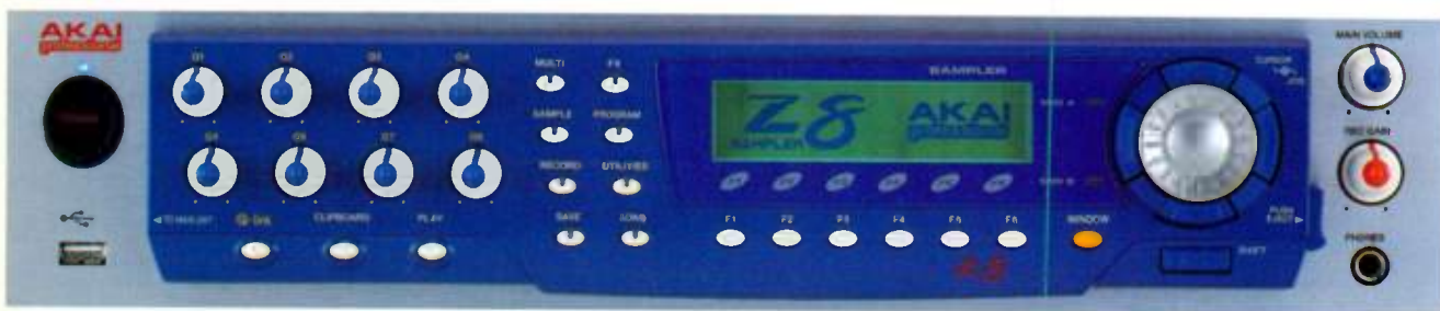
FIG. 1: With its detachable front panel and easy-to-access knobs, Akai's Z8 provides convenient control of synthesis parameters and effects. You can also use the knobs to tweak other hardware units.
