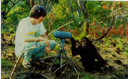
FIG. 13: Ruth Happel is using an MKH 30 and MKH 40 set up on a tripod to record a chimpanzee at Jane Goodall's research site, Gombe National Reserve, Tanzania.
