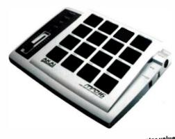
You can edit the Akai MPD16's MIDI parameter values using either the front-panel controls or the supplied MPD16 USB MIDI Pad Editor software.
