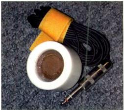
FIG. 14: This experimental hydrophone created by Rudy Trubitt and Bruce Koball places a piezo between two
