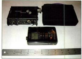
FIG. 2: Krause's main recording rig is very portable. Seen here are his Sony PCM-MI DAT recorder, Sound Devices preamp, and gel cell battery, which can run 18 hours on one charge.
