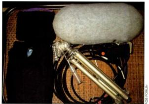
FIG. 3: Although Krause's entire recording rig (including a tripod and 10 meters of coaxial cable) fits into a backpack, it allows him to record for weeks at a time. His pair of Sennheiser microphones is inside the Rycote zeppelin.
