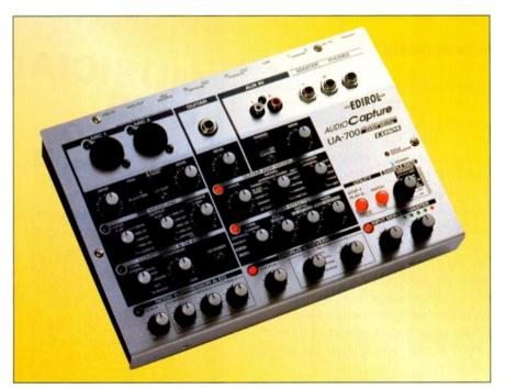
FIG. 1: The top panel on Edirol's UA-700 is packed with knobs, providing direct control over the microphone and guitar-amp modeling functions as well as the built-in effects.
