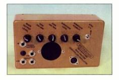
According to Metasonix, the TM-3's waveform is "very imperfect" and unlike waveforms produced by any other VCO. You can soft-sync the oscillators, forcing oscillator 1 to slave to oscillator 2. The TM-3 also offers a suboctave square wave that is one octave below oscillator 2, as well as brief pulses in the same octave as oscillator 2. Adjusting the Suboctave Stability control in conjunction with the suboctave waveform can produce inconsistent and unique effects.
