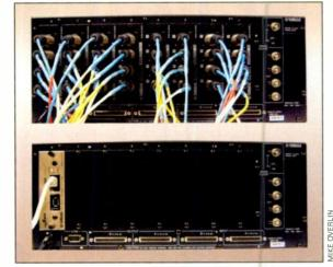
FIG. 2: One or two FireWire cables can replace many audio and MIDI cables. The top photo shows a typical rear panel (the I/O unit for Yamaha's PM1D mixer) without the benefit of FireWire or mLAN. In the bottom photo, the same rear panel is shown reconfigured with FireWire and mLAN.
