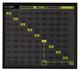
FIG. 1: FM7's Matrix display is used to route audio signals among the operators. Immediately after a patch has been initialized, it looks like this.
