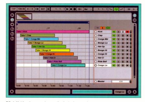
FIG. 4: Multitrack, tape-style recording in the Arrange view allows you to assemble complex arrangements from several input sources in one pass. Here, separate ReWire inputs from the ten pads of Reason's ReDrum drum sequencer were recorded in a single pass.
