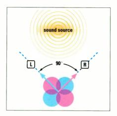
FIG. 2: A Blumlein pair specifies two figure-8 mics or capsules positioned so that the pickup axis of one is aligned with the null axis of the other. This stereo technique picks up sound equally, albeit in opposite polarity, from the front and rear.
