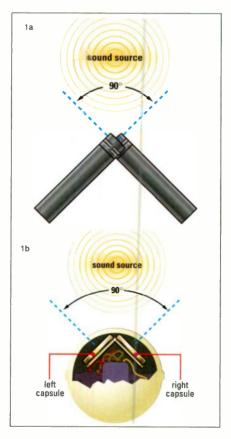
FIG. 1: The XY-coincident stereo-recording technique requires that the two capsules be positioned as closely together as possible. When using separate microphones, the best solution is an over-and-under configuration (Fig. 1a). Dedicated stereo mics, on the other hand, allow for the option of positioning the caps side by side (Fig. 1b).
