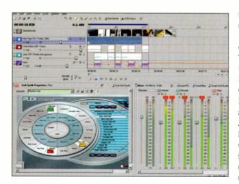
FIG. 1: Acid Pro 4.0a supports VST Instrument plug-ins and can trigger them from its new MIDI tracks. Note that each track type—video, MIDI, and audio—has its own icon, shown at the far left of each track.
