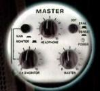
Assignable monitor / extra channel input with separate level control.
