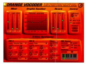
FIG. 3: The Orange Vocoder from Prosoniq features both sampled and analog-style carrier waveforms. With two oscillators, EQ, and reverb, it offers lots of tools for shaping sounds.
