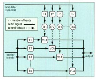
FIG. 2: The modulator is divided by a bank of bandpass filters (F), and then each band is analyzed by an envelope follower (EF). The carrier passes through a similar bank of filters. The control voltage (CV) of each EF controls the output level of the VCA on its corresponding carrier band. The modulated carrier bands are then recombined at the output.
