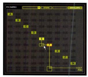
FIG. 2: To add frequency modulation (FM) in the Matrix display, simply click in the box shown and drag the mouse upward.
