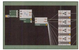
FIG. 2: To find the pitch class of a MIDI note in Reaktor, the MIDI note number (output by the NotePitch object) is divided by 12 in the Modulo object. The rest of the division is sent on to the author's stack of custom switching objects.
