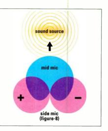
FIG. 3: The middle-side stereo technique employs a directional ("middle") mic aimed at the source and a bidirectional ("side") mic positioned to pick up sound coming from the sides. The signals must be properly demoded to create the final stereo image.
