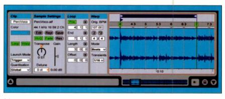
FIG. 3: Live's Clip view is where you choose the time-warping method as well as set various clip parameters. Here, a three-measure section of the audio clip has been selected for looped playback using the Beats method of time-warping.
