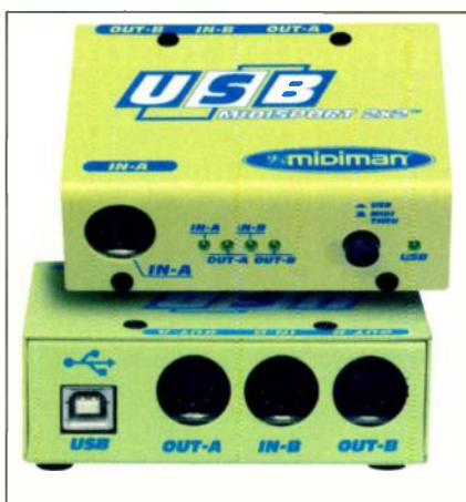
FIG. 1: To get MIDI in and out of your computer, you need a MIDI interface, such as this USB Midisport 2x2 from M-Audio. The Midisport has two outputs, which allow you to use up to 32 MIDI channels (16 on each output).
