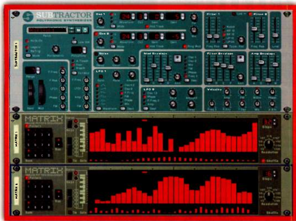
FIG 1: In addition to sending note data, Matrix Sequencers can be used to automate controls such as filter cutoff and volume. Here, Matrix 1 is sending note data to the Subtractor synth and modulating its filter-cutoff frequency, while Matrix 2 is controlling the Subtractor's amplitude.
