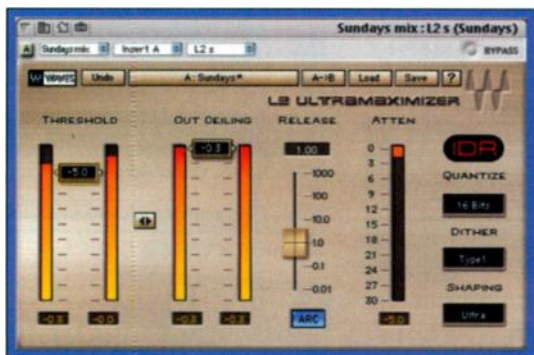
FIG. 4: The L2-Ultramaximizer plug-in's interface and operation are simple. Here, controls are set to produce an ultralow-noise, 16-bit CD master.
