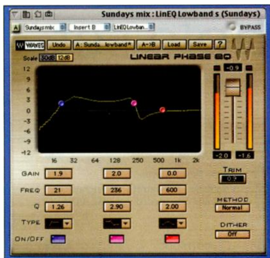
FIG. 2: This is a shot of the LinEQ Lowband plug-in illustrating a Resonant Hi-Pass filter at 21 Hz and a Resonant Low-Shelf at 236 Hz.
