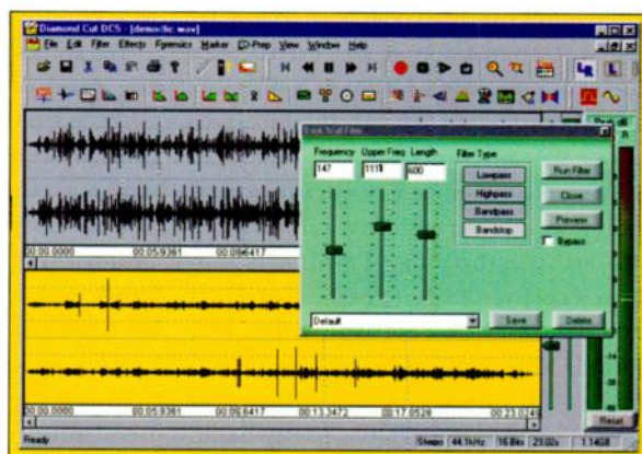
FIG. 10: Diamond Cut DC5 offers a full suite of denoising, click removal, and declipping tools. The display shows a scratchy file before and after a single pass through the declicking tool.
