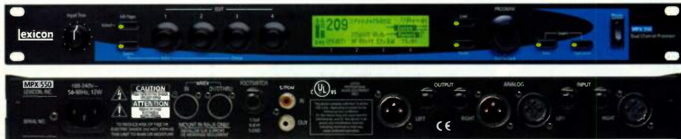
FIG. 1: The user interface (top) of the Lexicon MPX 550 is clean and simple. It features a large LCD screen and four soft knobs that make editing a snap. The rear panel (bottom) includes analog ins and outs on XLR and balanced \frac{1}{4} -inch jacks, digital S/PDIF on RCA coaxial jacks, and MIDI I/O.
