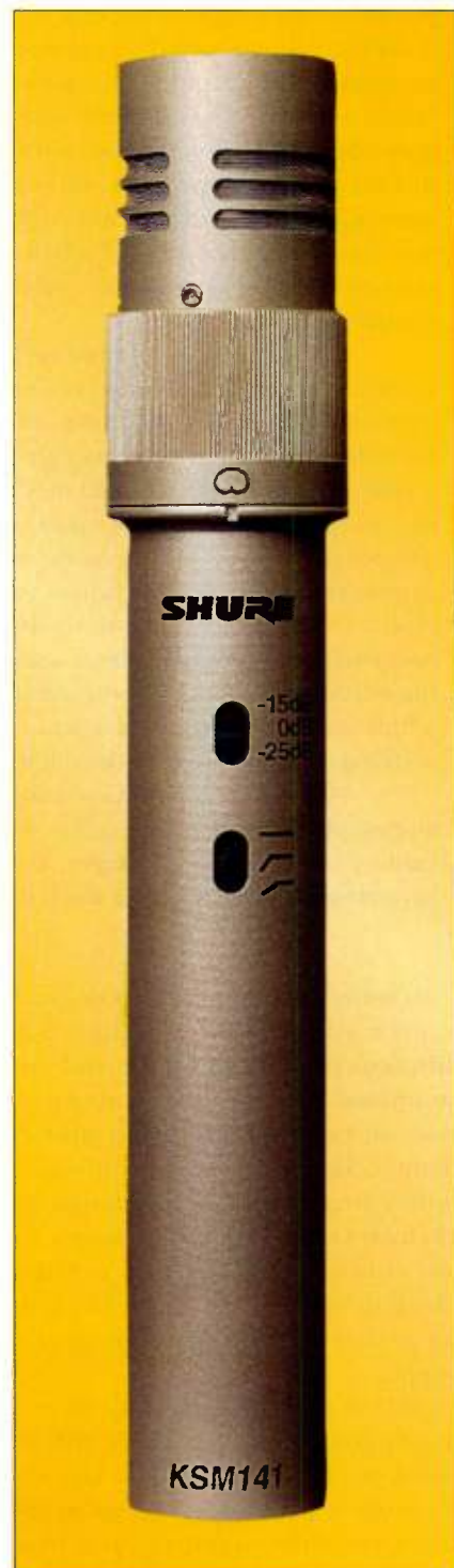
FIG. 1: The Shure KSM141 features a unique rotating ring used for mechanically switching the polar pattern. The mic offers cardioid and omnidirectional patterns, as well as dual-setting attenuation pads and highpass filters.
