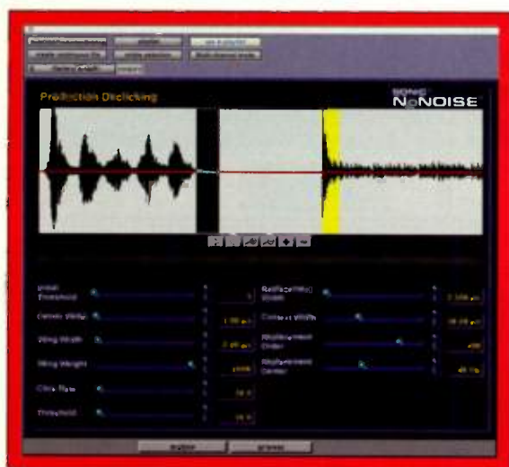
FIG. 7: The NoNoise Declicking module, as implemented for Pro Tools TDM or AudioSuite, provides automatic identification and removal of impulse noise artifacts.
