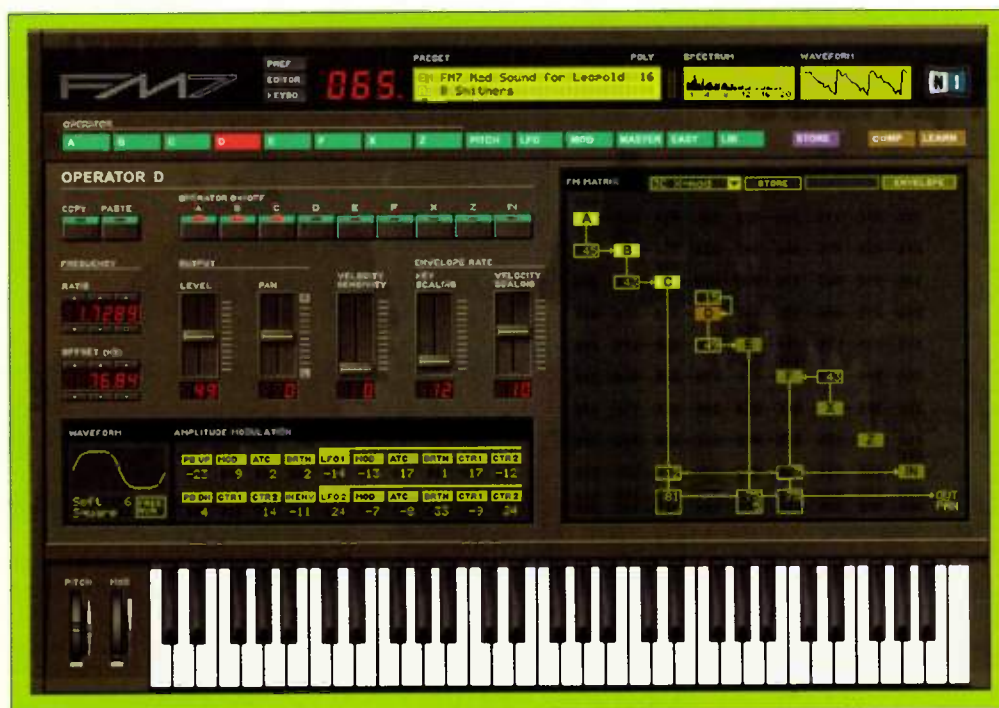
FIG. 1: In the right side of the window is the FM Matrix view, where the algorithm is defined in a simple click-and-drag interface. The arrows indicate signal flow, and the modulation amount can be adjusted by dragging your mouse on the displayed value.
