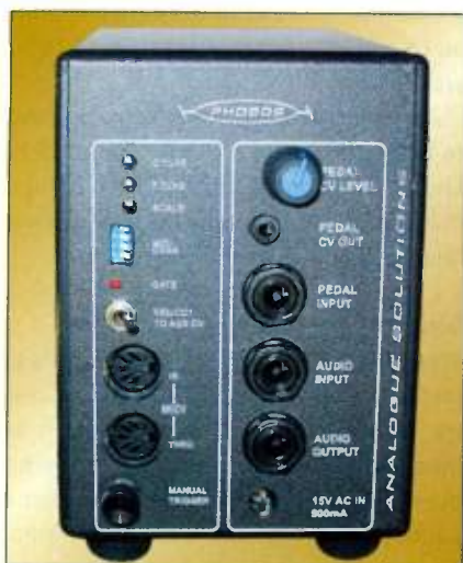
FIG. 1: The Black Coffee's rear panel includes MIDI In and Thru ports, a trigger button, and 1/4-inch jacks for audio input, audio output, and CV pedal input.
