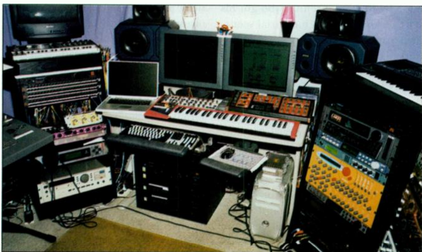
FIG. 1: Although Vrenna uses Pro Tools and an assortment of plug-ins and software synths, he also relies on hardware, including the Clavia Nord Lead synthesizer (the red keyboard, center) and the Waldorf MicroWave XT synth (the orange rackmount device to the right).
