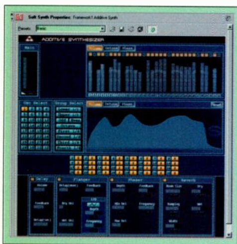
FIG. 1: Additive Synth is a VST plug-in that provides independent control of the amplitude and phase of up to 32 oscillators. Multiple oscillators can be grouped in various ways if, for example, you want to use the same envelope on the entire group.
