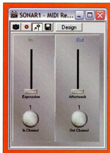
FIG. 4: Cakewalk Sonar's StudioWare Panel can map one MIDI message type to another. Here, it is receiving Expression on MIDI channel 1 and outputting Aftertouch on MIDI channel 1.
