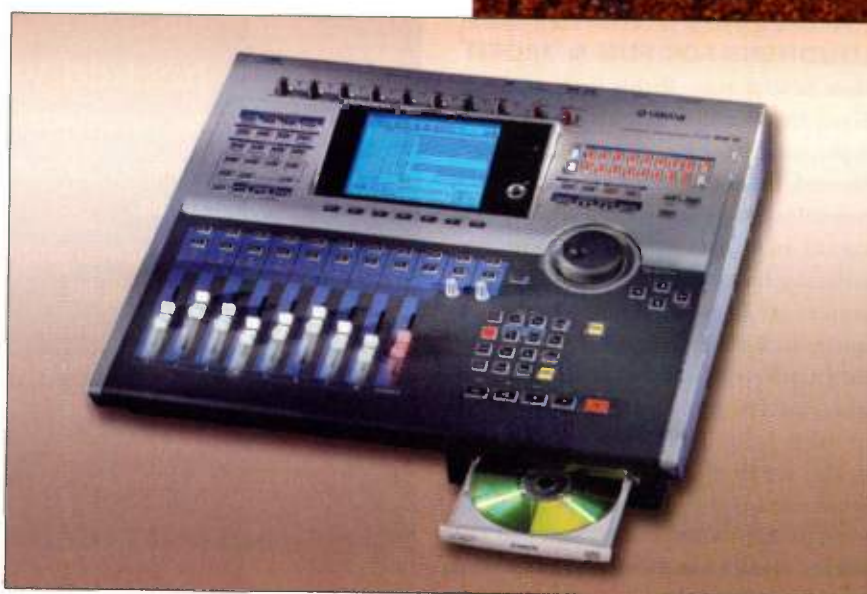
FIG. 1: The Yamaha AW2816 features a mixer with 28 inputs, 18 output buses, 9 motorized faders, and extensive automation; 24-bit, 16-track digital recording with a stereo master track; 2 multi-effects processors; and a built-in CD burner.
