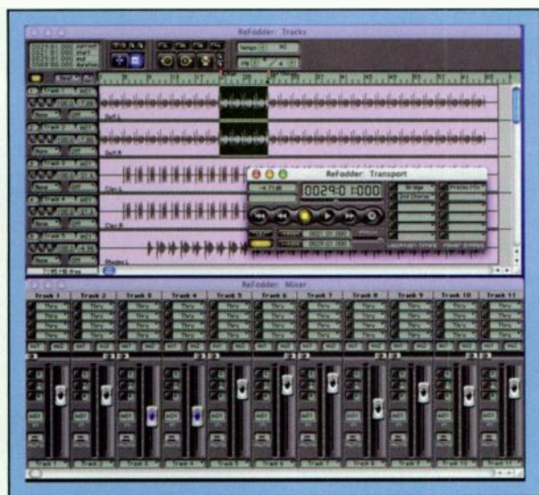
FIG. 1: Deck's Tracks window (top) can hold up to 64 playable tracks and 999 nonplaying Work tracks. The Mixer window's channel strips (bottom) provide a visual mixing surface. But aside from plug-in control, all of the Mixer's functions can be carried out in the Tracks window.
