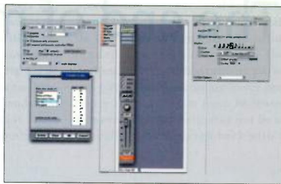
FIG. 5: In the Mixer Strip (Center) in Digital Performer's Mixing Console, incoming MIDI data passes through the transposition plug-in and then is fed to the arpeggiator. The windows surrounding the strip are the programming controls for the transpose function (left) and the arpeggiator (right).
