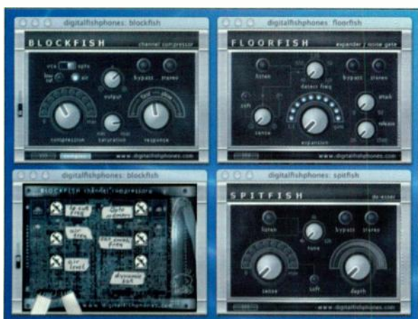
FIG. 7: The fish fillets channel insert package provides subtle analog-style dynamic processing and saturation. The front panel of BlockFish opens to reveal the circuit controls.
