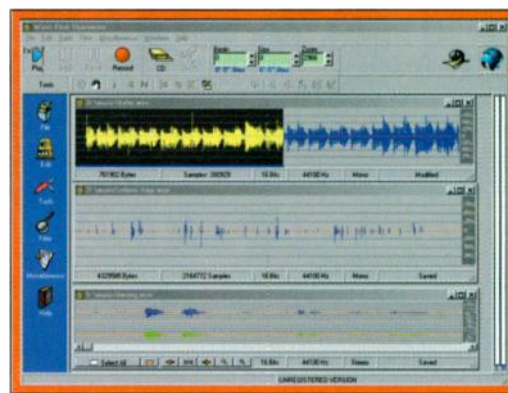
FIG. 10: Wave Flow is a stereo audio editor with a wide range of features. You can have as many files open at one time as you want.
