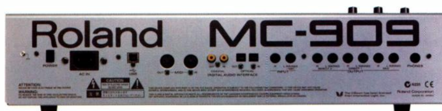
FIG. 2: In addition to its USB port, the MC-909's rear panel sports an array of I/O options, including MIDI, analog audio, and optical and coaxial S/PDIF.
