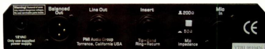
FIG. 2: Most of the VTB1's ins and outs are located on its rear panel, along with a switch for selecting mic impedance.
