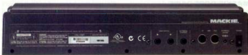
FIG. 2: The Mackie Control's spartan rear panel provides single MIDI In and Out ports along with two footswitch jacks and an External Control pedal jack.
