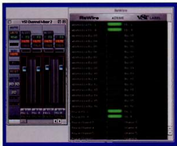
FIG. 2: The outputs of Propellerhead ReWire slave devices appear as inputs to the ReWire master device. In Cubase, activated inputs (green LEDs) appear as mixer channels (left).
