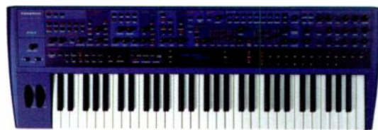
FIG. 4: The Supernova II Pro-X is Novation's flagship analog-modeling synth. It offers a profusion of front-panel controls, including 136 buttons that light up when they're active.
