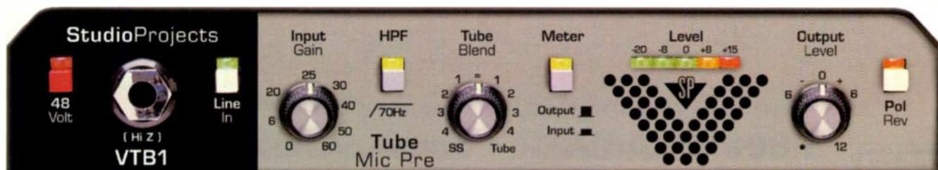
FIG. 1: The VTB1's almost primitive appearance only hints at its versatility. An instrument input and most controls are located on the front panel.
