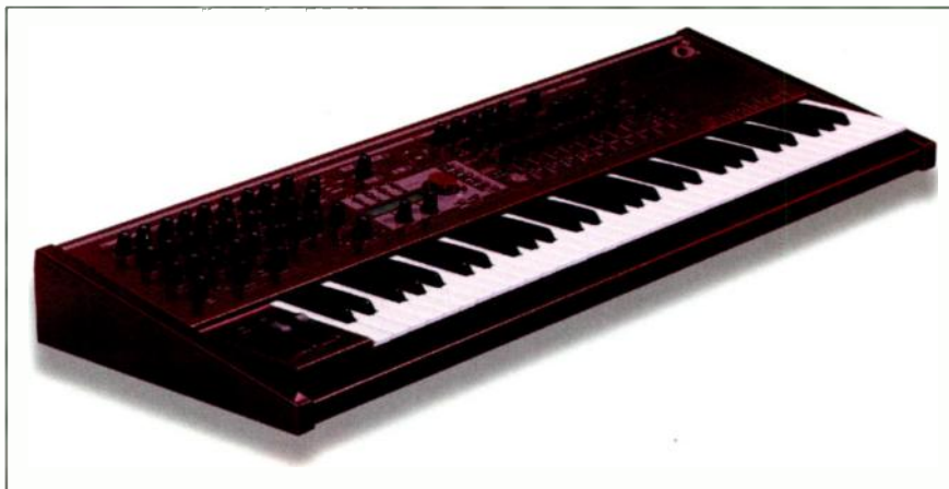
FIG. 10: The Waldorf Q+ differs from the original Q in that it has 16 real analog lowpass filters and dynamic voice management, which produces as much as 100-note polyphony.
