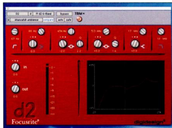
FIG. 4: IIR-based digital equalizers like Focusrite's d2 are efficient and widely used.
