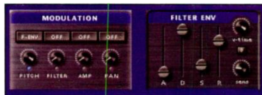
FIG. 4: In this figure, the F-ENV (Filter Envelope) is set to control the layer's Pitch Modulation control (left). The Attack time of the envelope (right) will control the pitch's slide rate, and the Sustain will control the actual sustaining pitch.
