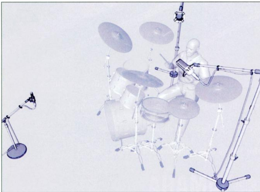
FIG. 3: The minimalist drum-miking setup made popular by engineer Glyn Johns (of Led Zeppelin fame) requires only three mics: one directly in front of the kit, and a spaced pair of matching overheads behind, each aimed at the snare drum.
