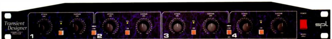
FIG. 1: The Transient Designer 4 uses VCAs controlled by envelope generators to process dynamics independent of levels.
