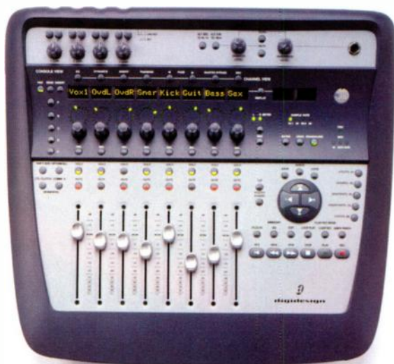
FIG. 1: Digidesign's Digi 002 is notable for its well-designed control surface and its integration with Pro Tools LE, which comes with the interface.
