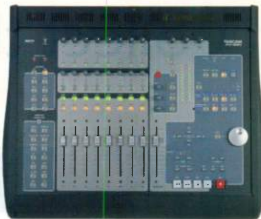
FIG. 8: Tascam's new FW-1884 is currently the largest of the FireWire interfaces. It sports a full-featured control surface with a 4-port MIDI interface. The FW-1884 is designed to support a number of DAW applications.
