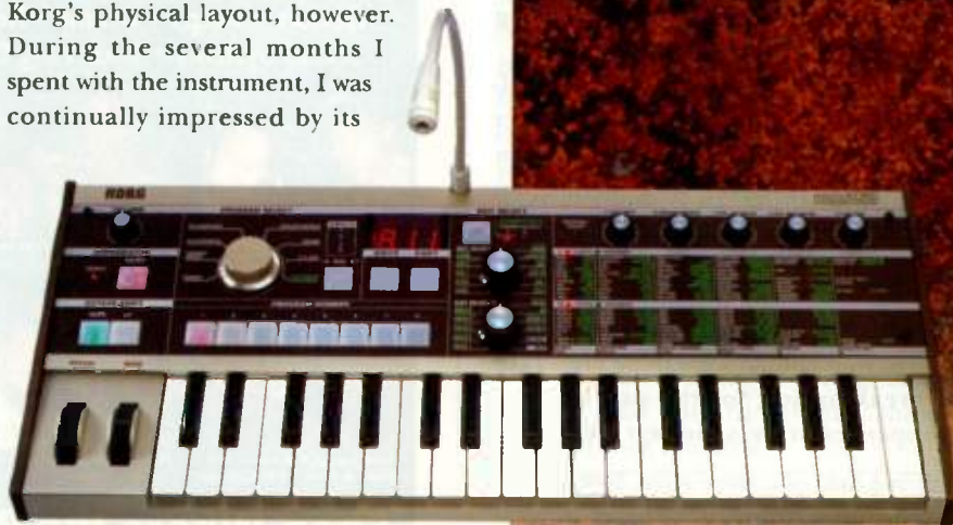
FIG. 1: The MicroKorg delivers the enormous sound of Korg's MS2000 in a lightweight, battery-powered box less than 21 inches wide. Its five control knobs work with two 11-step selector knobs to adjust nearly 200 parameters.
