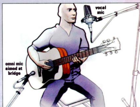
FIG. A: One successful method for miking a singing guitarist involves using an omnidirectional mic placed close to the bridge or sound hole. The vocal mic is positioned slightly above and off to the side of the singer's mouth.
