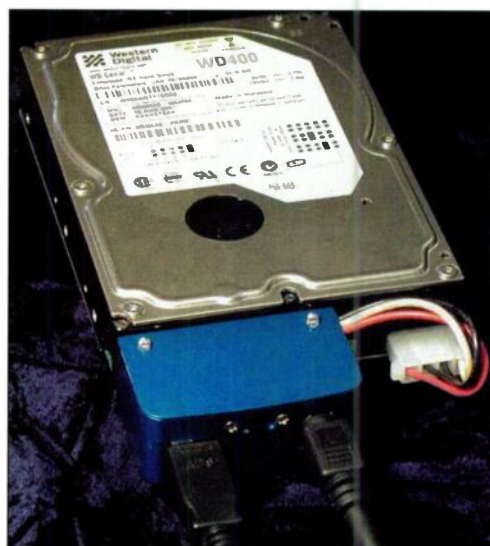
FIG. 2: WiebeTech makes the utilitarian DriveDock line of FireWire adapters, allowing you to hook up off-the-shelf bare drives to an IEEE 1394 connection.
