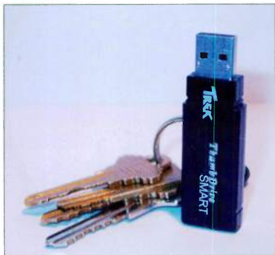
FIG. 3: Trek's ThumbDrive is one of the many solid-state USB storage devices to hit the market recently. Though its speed isn't up to the needs of multitrack audio recording, its convenience for storing samples and song ideas is undeniable.
